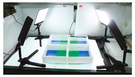
Figure A1. Instrument setting used to perform the color preference test in zebrafish.
