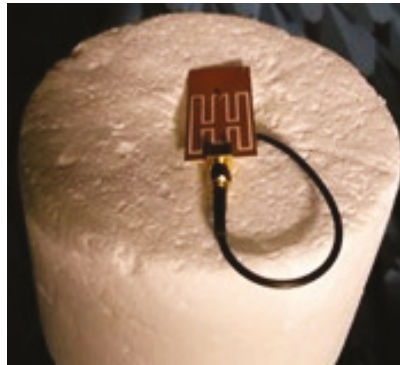
Figure 9. Antenna’s farfield measurement setup.
