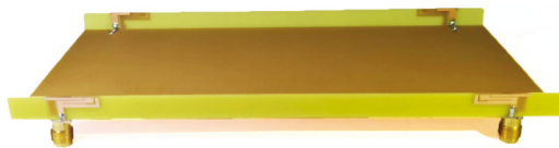
Figure 6. Photograph of the fabricated antenna prototype.
