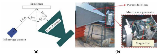
Figure 14. MWT setup (a) and Horn (b) in University Institute of Technology of Bethune [56]. Reprinted/reproduced with permission from Scientific Research Publishing Inc.
