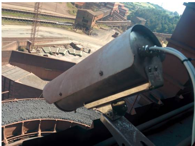
Figure 13. Infrared camera for sinter monitoring.
