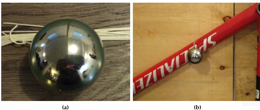
Figure 4. Calibrated steel ball used in the experiments. (a) Steel ball and rod. (b) Ball hitting a similar bicycle frame to produce impact damage.
