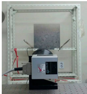
Figure 7. Location of the fixed target specimen during scanning.
