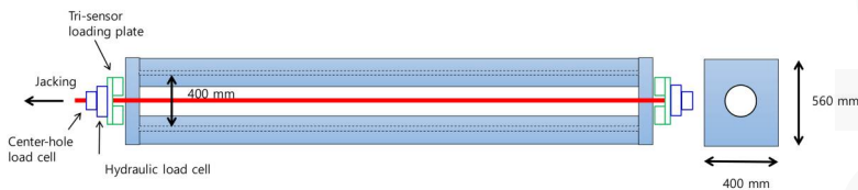
Figure 2. Steel frame of a girder for validation test (not to scale, stiffeners not shown).
