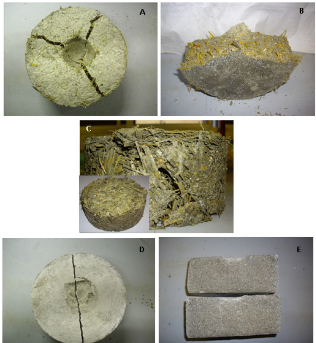
Figure 12. Samples after the impact test. (A,B) S3 sample, (C) S3C sample, (D,E) perlite sample.
