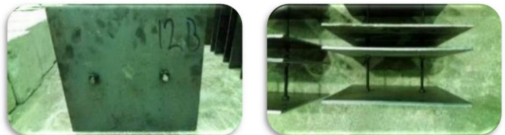
Figure 3. Reinforced plates with stud-bolt connectors.
