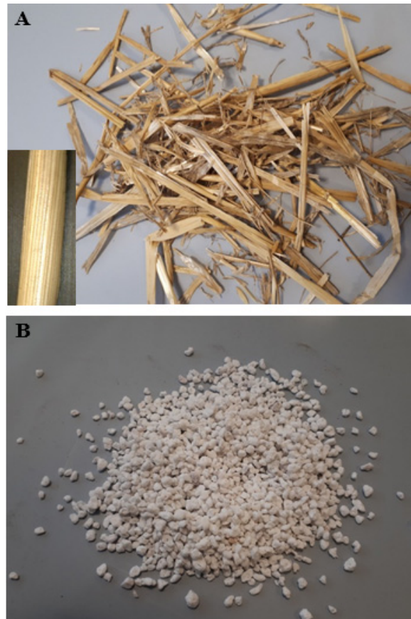
Figure 1. (A) Straw before use and, in the inset, after cutting. (B) Perlite beads.
