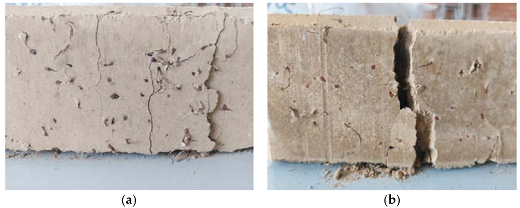
Figure 9. Tested soil–cement WTSF blocks: (a) 0.75% WTSF and (b) 1.50% WTSF.
