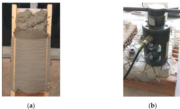
Figure 3. Application of fiber-cement mortar on the substrate of an aerated concrete block (a); demonstration of testing the adhesion of fiber-cement mortar to the substrate (b).
