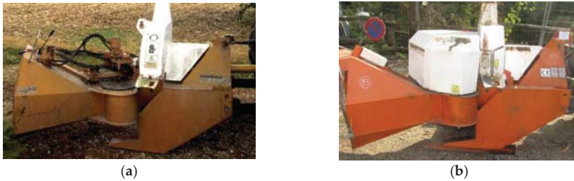
Figure 6. Specimens of the same model of wood chipper manufactured in different years on which lacked feeding area identification and safety pictorials were worn or incomplete. Moreover on (a) the hydraulic components are freely accessible while in (b) they are housed in a metal protection case.
