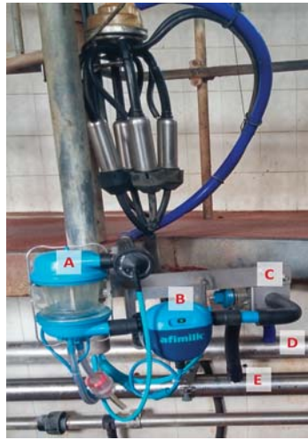
Figure 1. The Afilab (B), installed next to the AfiMilk (A) milkmeter at each milking unit, performs real-time analysis of milk components using spectroscopy in the near infrared. Milk with predefined coagulation properties is separated and conveyed, thanks to controlled valves (C), through two different milklines (D or E) in a predetermined cooling tank.
