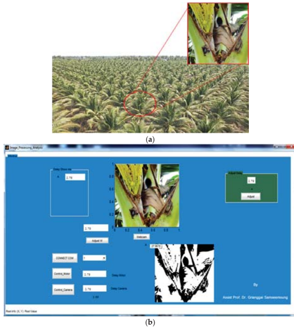
Figure 5. Image from the remote monitoring system; (a) coconut pest disease infestation, (b) image data processing (segmentation).
