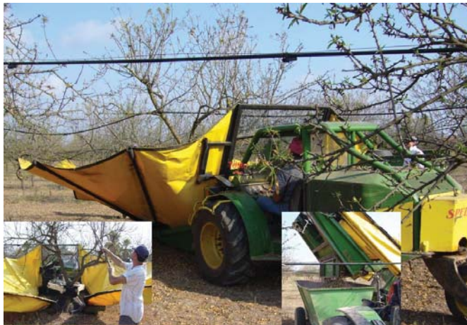
Figure 2. Self-propelled harvester SICMA Ltd., model "Speedy"; inset shows the manual pole beating for residual product.
