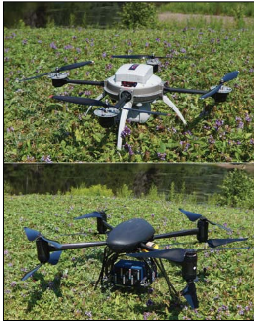
Figure 5. Two unmanned aerial system (UAS) quadcopters deployed by Nipissing University researchers for agricultural monitoring. The Aeryon Scout (Aeryon Labs Inc., Waterloo, ON, Canada) carries an infrared ADC lite camera (Tetracam, Chatsworth, CA, USA), whereas the Dragan Flyer X-8 (Draganfly Innovations Inc., Saskatoon, SK, Canada) carries a Mini-MCA camera (Tetracam, Chatsworth, CA, USA).
