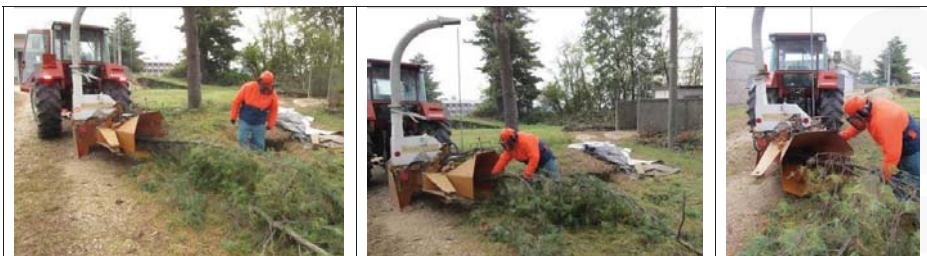
Figure 7. Images of the procedures followed during the wood speed test, operated with a 28-years-old wood chipper.
