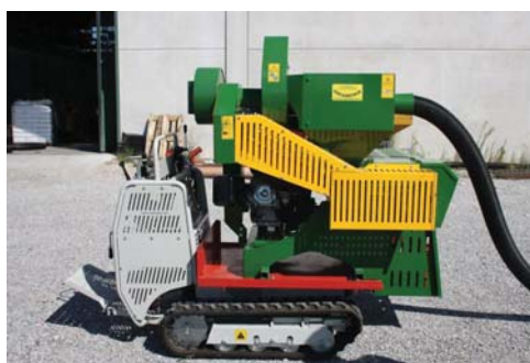
Figure 1. Photo of the small-scale machine for nuts harvesting proposed in the study of [44].
