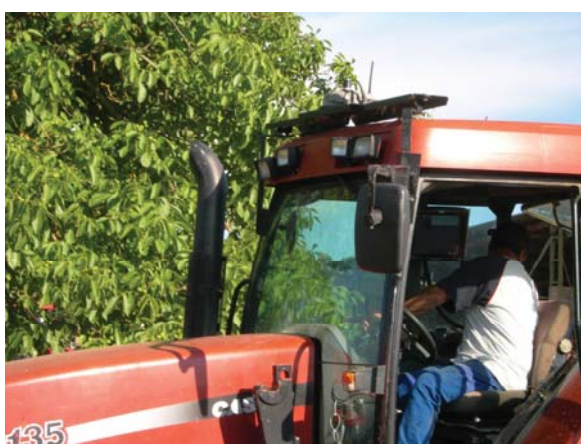
Figure 2. Monitor and antenna installed on the tractor.
