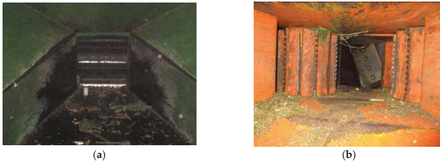
Figure 1. Detail of infeed components (rollers) (a) and knife on the disk shaft (b) of the surveyed in-use wood chippers.
