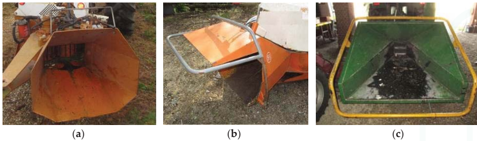
Figure 3. Some examples of protective devices that do not comply with standard requirements. (a) This machine presented no safety devices around the edges of infeed chute. (b) Side and upper protective devices were present, but there was no lower protective device (mandatory for the standard). (c) The infeed chute was equipped with side, lower and top protective devices, but in order to comply with the safety standard draft, the top protective bar should have a separate control or be replaced by an emergency stop.
