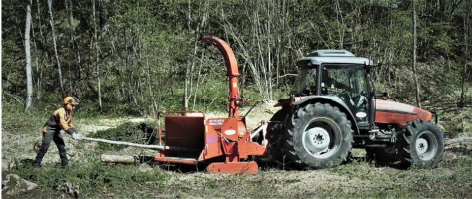
Figure 1. Manually fed wood-chipper used in a riverbank vegetation clearing cut.
