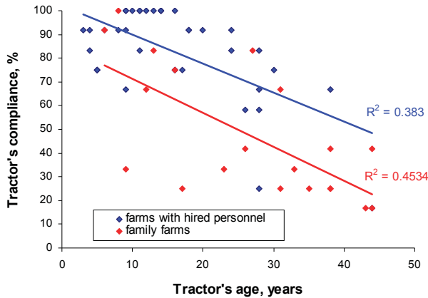
Figure 5. Tractor’s compliance (% of compliant items) vs. tractor’s age (years) in farms with or without hired personnel.
