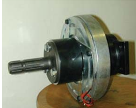
Figure 3. Decoupling system installed between power outlet and cardan shaft.
