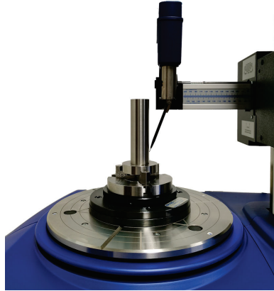
Figure 3. The roundness and cylindricity errors measurement process.
