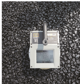
Figure 4. PQI380 used in in-situ test.
