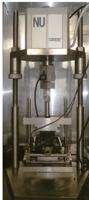
Figure 4. ITSM test setup.
