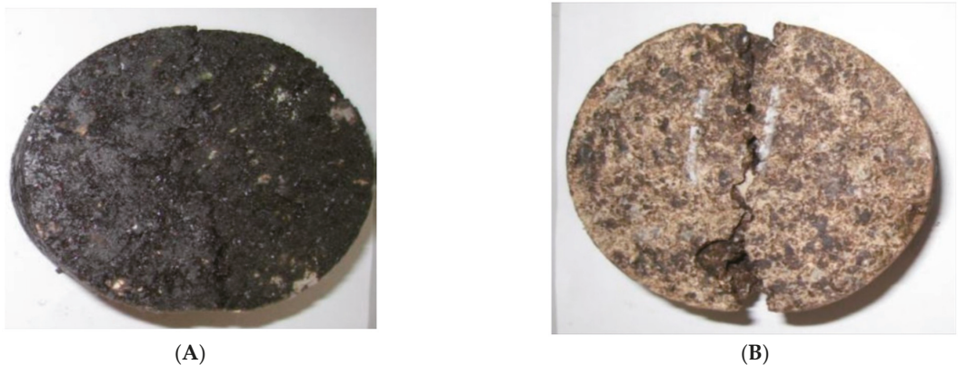
Figure 14. Cold recycling asphalt mixture (A) Emulsified asphalt cold recycling, (B) Foam cold recycling.
