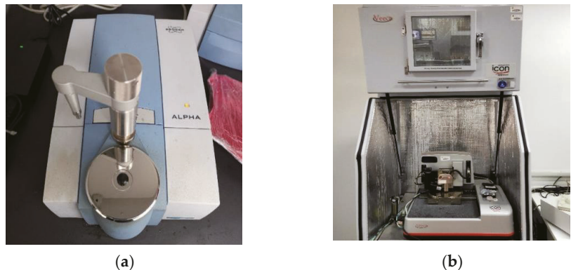
Figure 3. Microscopic analysis equipment: (a) FTIR-ATR; (b) AFM.
