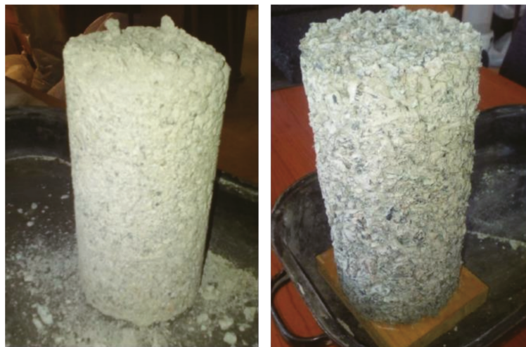
Figure 5. Specimens for CTT: GM 0/22 (left); GM 0/32 (right).
