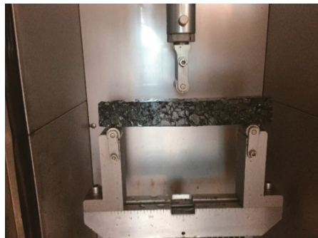
Figure 8. Bending test of specimen.
