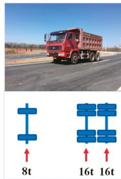
Figure 3. Axle load and axial distribution of trucks in loading mode I.
