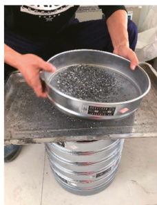
Figure 2. Aggregate and limestone powder screening.
