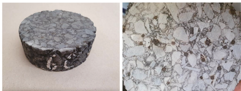
Figure 6. Image of 10 mm SMA—mix 6 containing 1.45% capsules in the mix.
