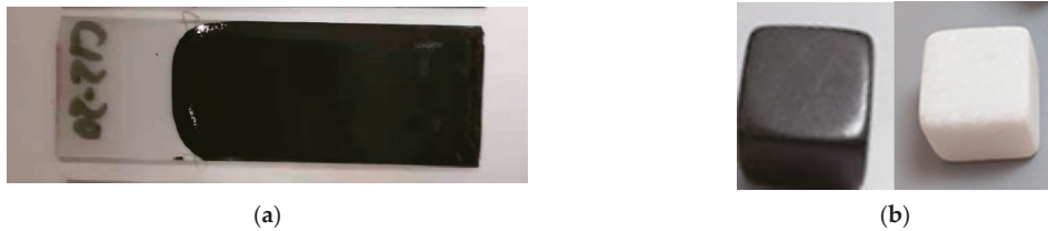
Figure 2. Contact angle measurement sample: (a) Crumb rubber sample, (b) Basalt and limestone blocks.
