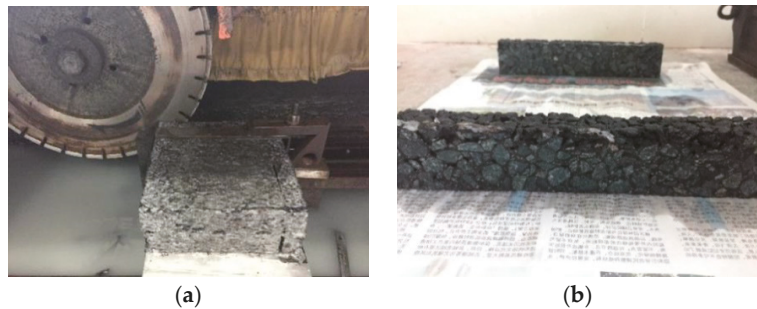
Figure 7. (a) Fabrication of prismatic specimen; (b) prismatic specimen prior to testing.
