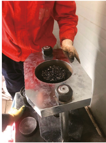
Figure 5. Demoulding process of Marshall test specimens.
