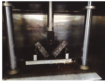
Figure 4. Three-point bending test of recycled asphalt mixture.
