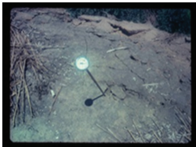
Figure 8. Peat fires at depth were a common result of the drainage of the Hula valley swamps in Israel. The temperature probe in the residual ash reveals prolonged sub-surface burning. Source: Edward Maltby.
