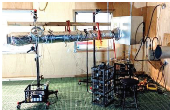
Figure 2. Test stand configuration and DAQC system in ADL for DGFCH test.
