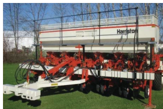
Figure 16. Harriston Clamp potato planter. Reprinted with permission from ref. [96]. Copyright 2020 Harriston Industries.
