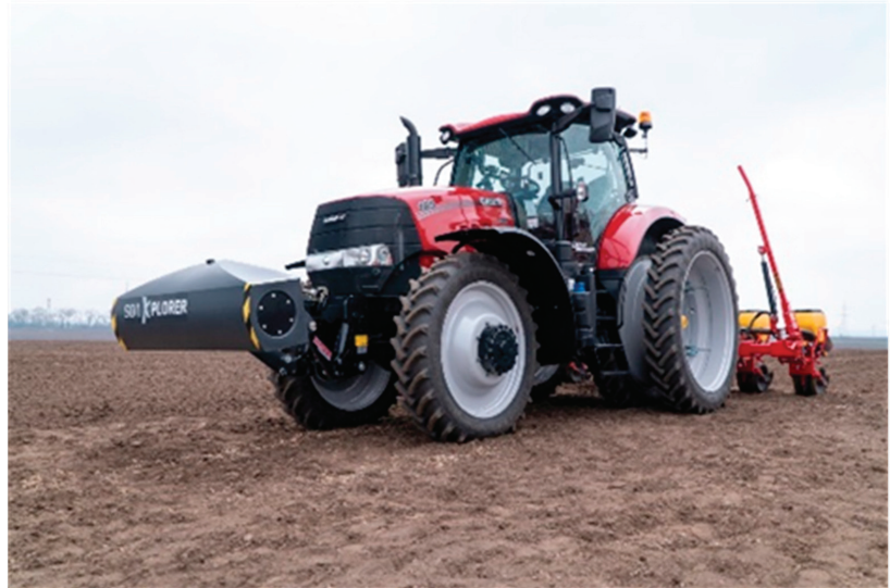
Figure 12. SoilXplorer device for measuring soil structure differences [60].
