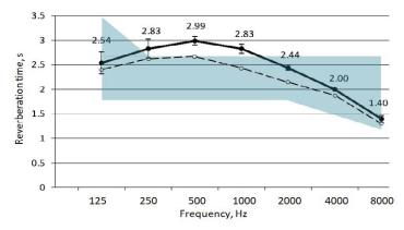
**Figure 8.** The reverberation time of the winter garden. Continuous line and numerical values: acoustical measurements (the average of 8 observation points, room without public). Measurements were made in accordance with the ISO 3382-2 standard [22], sound source—pistol shot. Dashed line—reverberation time taking into account the presence of the audience, choir and orchestra, see Appendix A. The range of recommended values of reverberation time for the occupied room is marked in blue [17].
