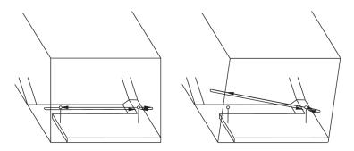
Figure 9. Shifting the zone of flutter echo formation (left) above the level of the performers' heads by deviating the side walls from the vertical (right).
