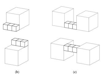
**Figure 4.** Typology of the all-glass structure by functional-spatial aspects: (**a**) pavilions; (**b**) extensions; and (**c**) links (figures by the author).
