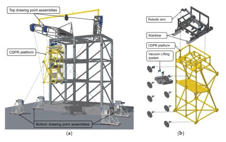
Figure 6. (a) Design of the Hephaestus cable-driven parallel robot (CDPR) prototype; (b) detailed depiction of the modular end-effector of the CDPR system.
