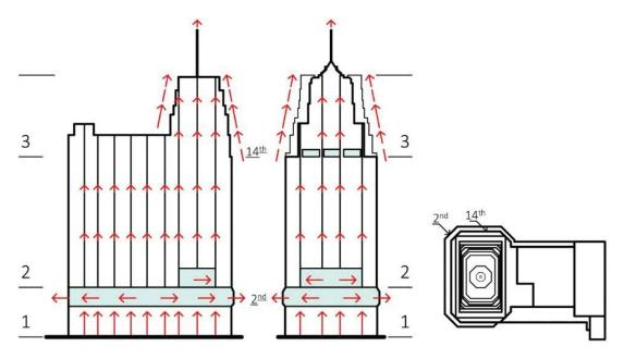
Figure 18. JSS Building-tripartite scheme and gradually decreasing plan, scheme of tension lines.
