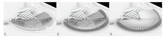
**Figure 11.** Stages of the conversion of the amphitheater into the odeon in Biała Podlaska. (1) Existing amphitheater with roof over the stage. (2) New steel space truss on the crown of the fortification ramparts. (3) New membrane roof with tensioned surface forming cables. Author graphics based on source BP Projekt.
