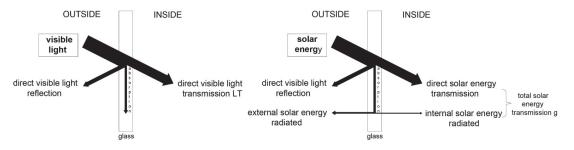
**Figure 3.** Schematic of the transmission of visible light and solar energy through glass panes (figure by the author).
