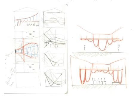
Figure 6. (a) The early canopy design concept based on graphic statics describing how to use compression element in the center and tension elements on both sides to create a covering surface; (b) Sketches of the canopy's different hanging methods according to different functional use.
