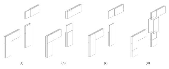
Figure 19. The types of connection glass layers in frames nodes: (a) tongue and groove; (b) tongue and groove; (c) single lap; and (d) cover layers (developed by the author based on the [99]).
