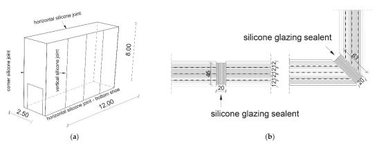
**Figure 27.** The Apple Retail Store in Milan: (**a**) axonometry with marked silicone joints; (**b**) detail of the connection of glass panes in the wall and the pavilion's corner (developed by the author based on the [113]).
