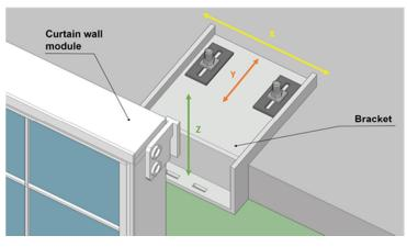
Figure 4. Schematic diagram of a typical bracket on the concrete building floor and its connection with a CWM module (the drilling technique).
