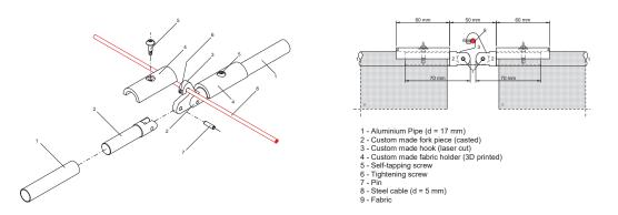
Figure 12. The structural detail drawings of the fabric, pipe, and cable connections.
