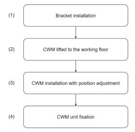
Figure 3. Four main steps in the curtain wall module (CWM) installation.
