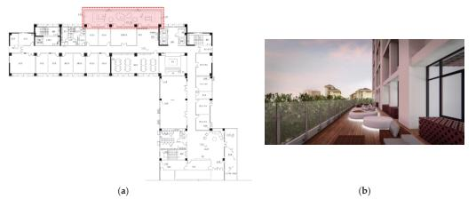
Figure 7. The third-floor terrace after optimal design. (a) Optimized plan. (b) Rendering of the space after optimal design.
