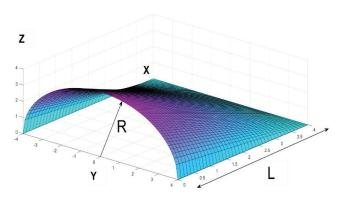
**Figure 2.** Explanation of the parts of a straight conoid with circular directrix, in this case R = L = 4.
