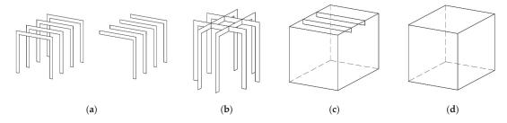
Figure 18. Typology of glass structural systems used in all-glass objects: (a) frames; (b) grillages; (c) beam-wall systems; and (d) plate-wall systems (figures by the author).
