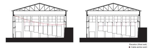
**Figure 8.** (a) Spanning the cables along the short side of the building would have called for a secondary structure to keep the top part of the fabric strips on the same height; (b) Conversely, when the cables span the longitudinal direction, it is possible to avoid the need for this secondary structure.
