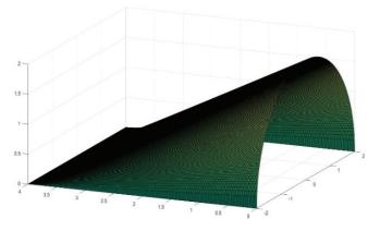
Figure 7. The single conoid limited by a rectangular plane and semicircle.
