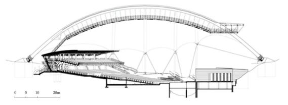
Figure 7. The scale of the main foundations of the load-bearing arch structure Forest Opera House in Sopot cross-section. https://inzynierbudownictwa.pl/stalowa-konstrukcja-z-motylim-dachem/10.05.2021 (accessed on 16 July 2021).
