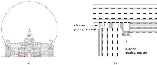
Figure 26. The underground station Dilworth Park in Philadelphia: (a) form of pavilions (© Kieran-Timberlake), (b) detail of roof plate–wall connection (developed by the author based on [112]).
