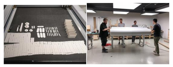
**Figure 14.** (a) The 3D-printed and laser-cut elements for the joints (Photo by Alessandro Tellini); (b) The rolling machine for measuring the fabric strips and for the installation of the pipes developed at the Raplab (ETH Zurich) (Photo by Giulia Boller).
