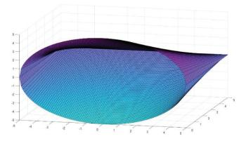
Figure 6. The second radiation principle of Cabeza-Lainez applied to the form-factor of a double conoid.
