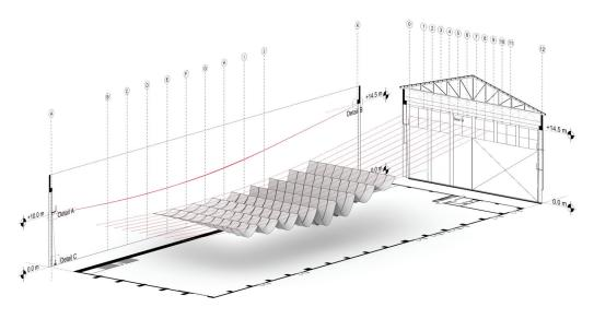
**Figure 9.** Axonometric diagram of the relationship between the structural model and the order of the existing building. In its final configuration, the cables were suspended along the building's longitudinal axis, thus eliminating the secondary structure and giving more freedom for the placement of anchor points on the walls.
