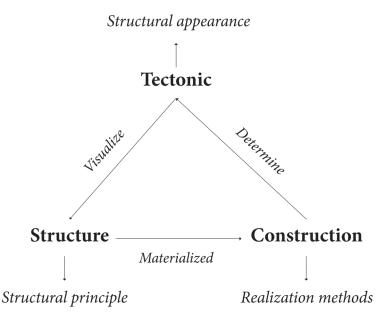
**Figure 5.** The graphical representation of the relationship between Structure, Construction, and Tectonic from the concept of Eduard Franz Sekler.
