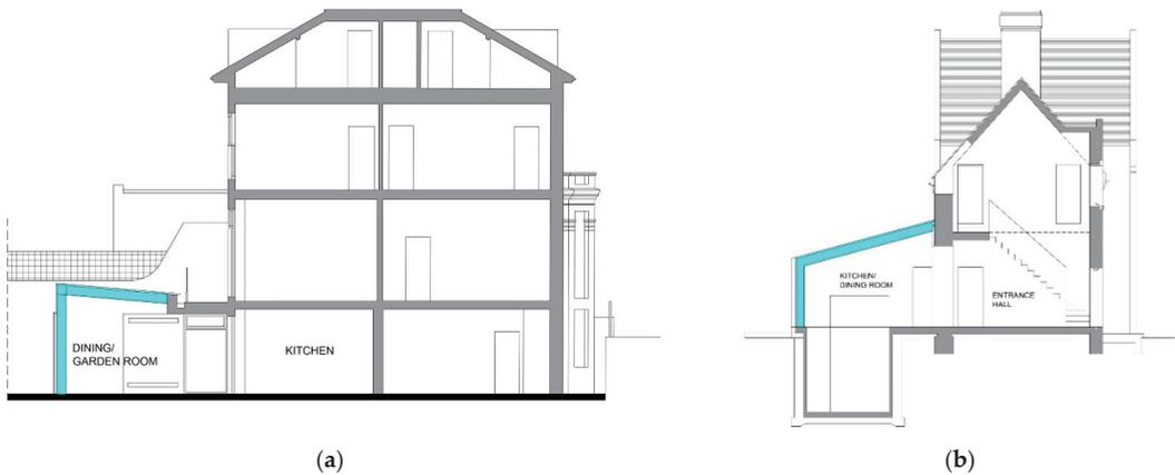
**Figure 7.** Extension in houses: (a) house at Castelnuau in London (developed by the author based on the architect's drawings); (b) house at Milnthorpe Corner in Winchester (developed by the author based on the architect's drawings).
