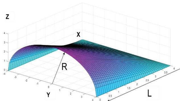
**Figure 2.** Explanation of the parts of a straight conoid with circular directrix, in this case  $R = L = 4$ .
