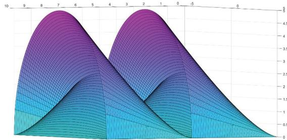
Figure 29. Outline of proposed skylights with internal conoid glazing.
