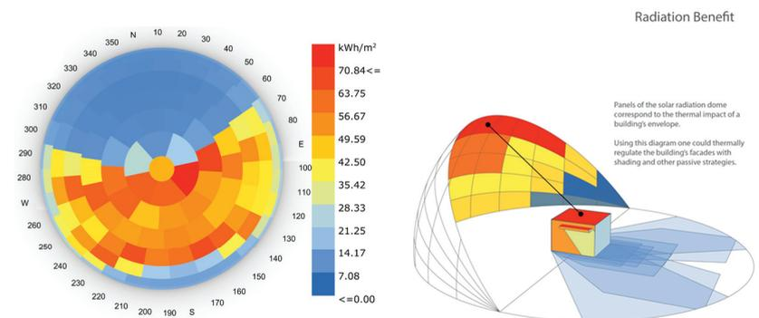
Figure 5. Sun radiation diagram.
