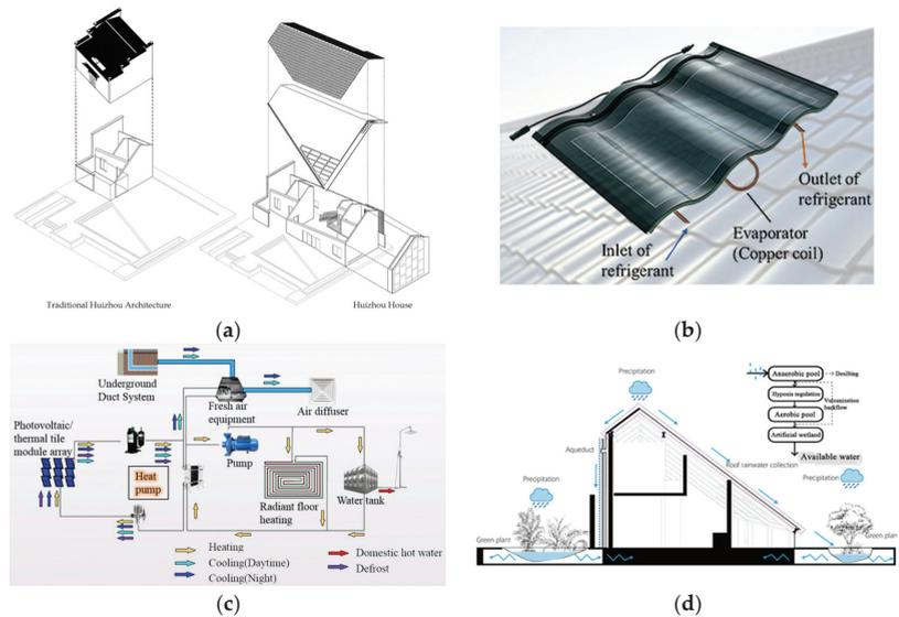
**Figure 8.** Main results of the HUI House. (a) Modern Huizhou architecture. (b) Solar chips. (c) Multi-functional supplying system. (d) Rainwater use system.
