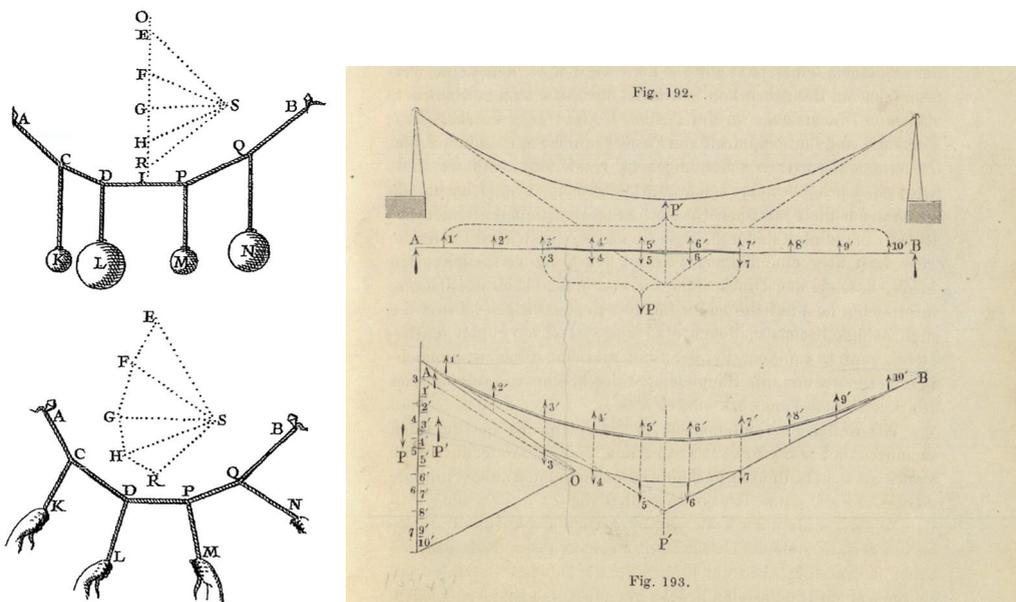
**Figure 4.** (a) Stevin's diagrams illustrating equilibrium states for a cable under different loads, and the corresponding internal forces using graphic statics [16]; (b) Culmann's introduction of the polygon of forces and funicular polygon [18] (p. 513).
