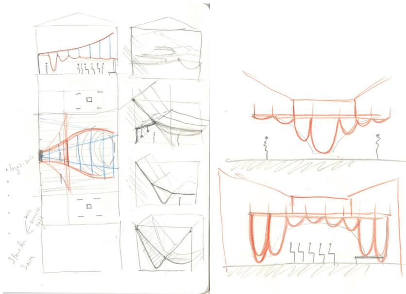
**Figure 6.** (a) The early canopy design concept based on graphic statics describing how to use compression element in the center and tension elements on both sides to create a covering surface; (b) Sketches of the canopy's different hanging methods according to different functional use.
