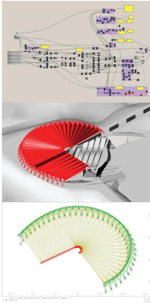
A. A parametric script, made to find a form in existing historical environment. Controls, roof surfaces density, geometry of external structure, heights cables mounts on building.
