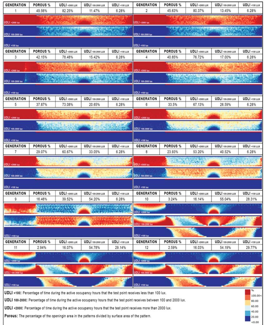
Figure 26. Daylighting analysis of the pattern generations.
