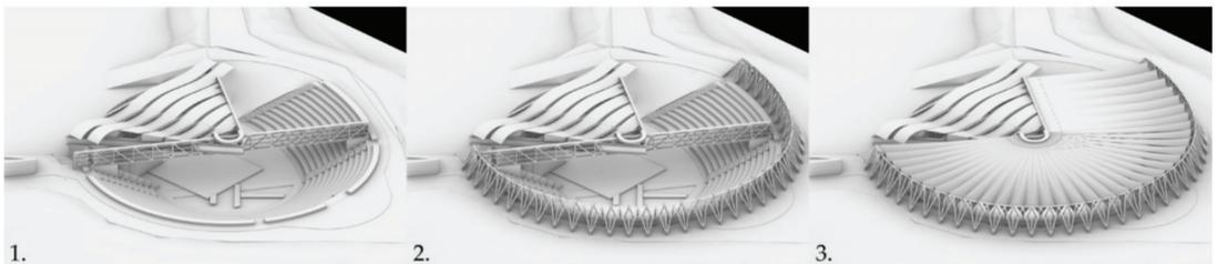
Figure 11. Stages of the conversion of the amphitheater into the odeon in Biała Podlaska. (1) Existing amphitheater with roof over the stage. (2) New steel space truss on the crown of the fortification ramparts. (3) New membrane roof with tensioned surface forming cables. Author graphics based on source BP Projekt.
