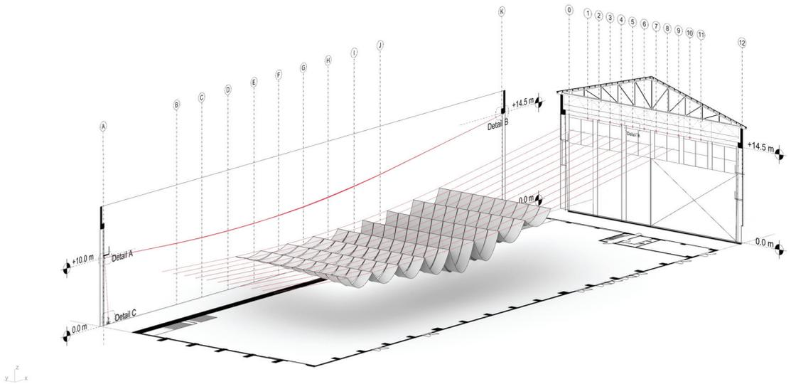
**Figure 9.** Axonometric diagram of the relationship between the structural model and the order of the existing building. In its final configuration, the cables were suspended along the building's longitudinal axis, thus eliminating the secondary structure and giving more freedom for the placement of anchor points on the walls.
