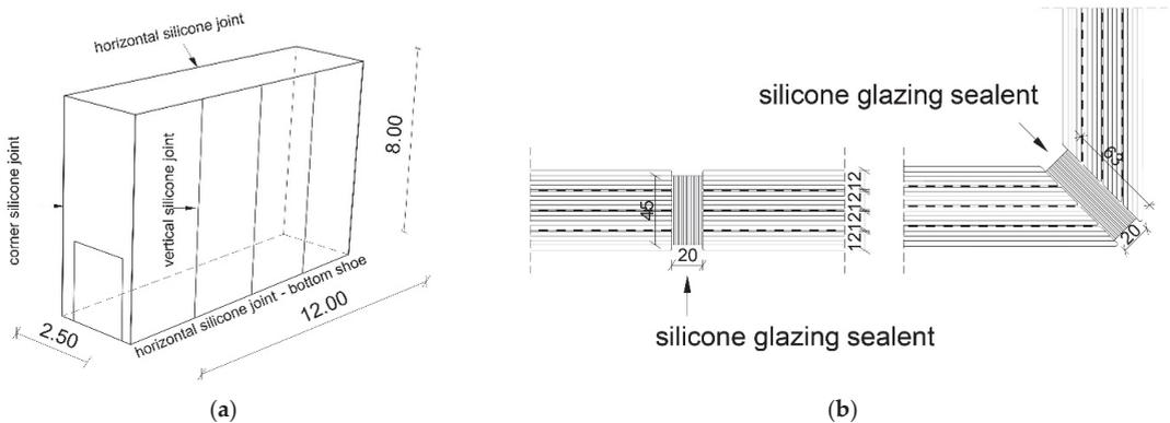
**Figure 27.** The Apple Retail Store in Milan: (a) axonometry with marked silicone joints; (b) detail of the connection of glass panes in the wall and the pavilion's corner (developed by the author based on the [113]).
