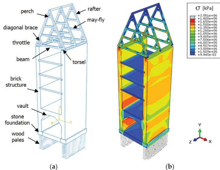
**Figure 2.** Medieval tenement house in Gdańsk: (a) numerical model and description of the structural members, (b) results of maximum stress maps in (kPa).
