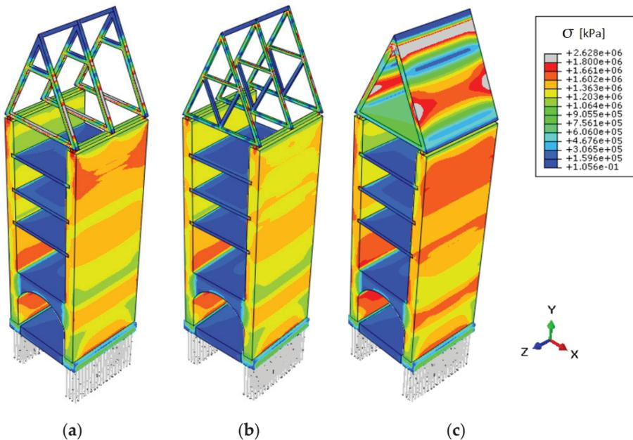
Figure 13. Numerical model of roof structures of modern tenement houses in Gdańsk: (a) wooden rafter framing of one piece, (b) steel rafter framing, (c) roof made of reinforced concrete slabs; stresses in (kPa).
