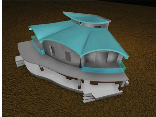
**Figure 25.** Three rotated conoidal roofs designed for a musicians' family. Sanlucar (Seville).
