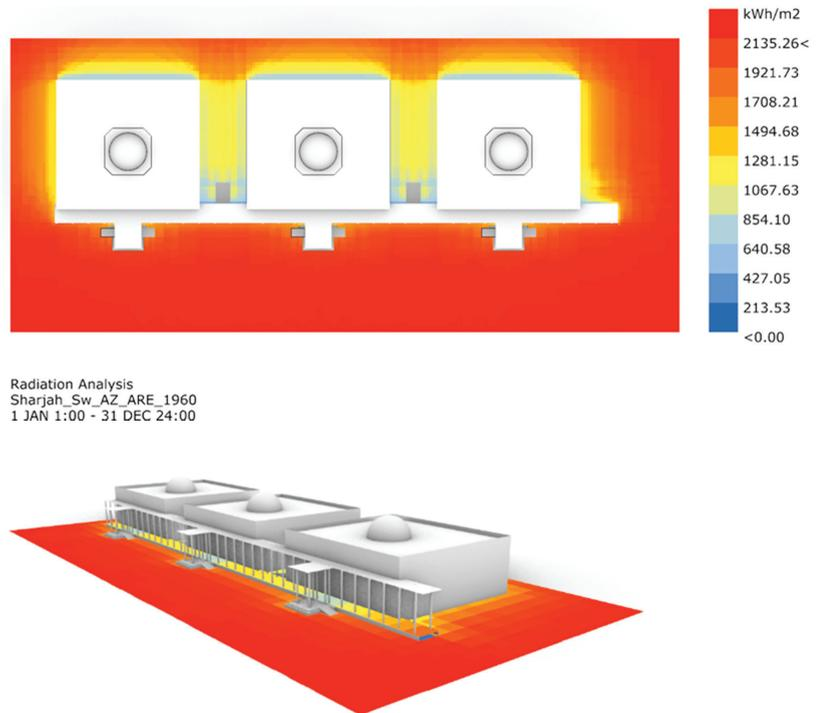
Figure 20. Cumulative solar radiation analysis.
