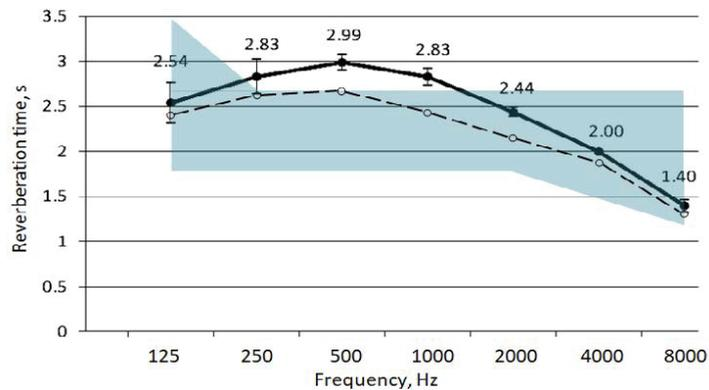
**Figure 8.** The reverberation time of the winter garden. Continuous line and numerical values: acoustical measurements (the average of 8 observation points, room without public). Measurements were made in accordance with the ISO 3382-2 standard [22], sound source—pistol shot. Dashed line—reverberation time taking into account the presence of the audience, choir and orchestra, see Appendix A. The range of recommended values of reverberation time for the occupied room is marked in blue [17].
