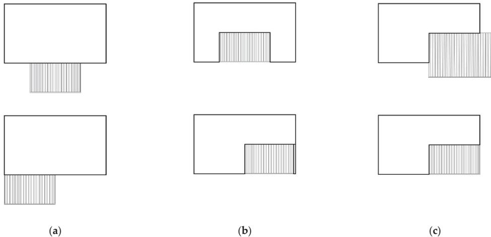
**Figure 6.** Extension in houses: (a) placed outside the building floorplan contour; (b) placed inside the building floorplan; and (c) placed in the corner (figure by the author).
