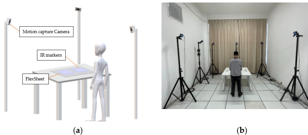
Figure 1. Composition and operation of deformation input: (a) Deformation input environment diagram; (b) Experiment with OptiTrack and FlexSheet.
