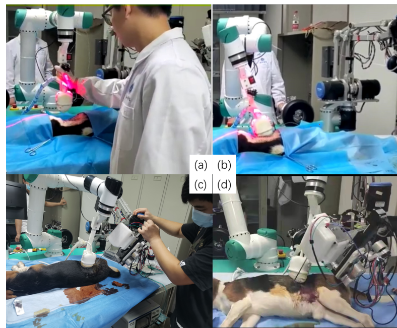
Figure 18. Process of the animal tests. (a) US arm docking operation; (b) master–slave control of US arm for image guidance; (c) puncture arm docking operation; (d) the surgery process of the animal test.
