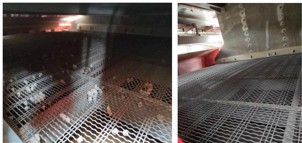
Figure 12. Photographs showing the condition of sieve blockage with difficult grains: At a toss index of 5.5 (left), at a toss index of 6.6 (right).
