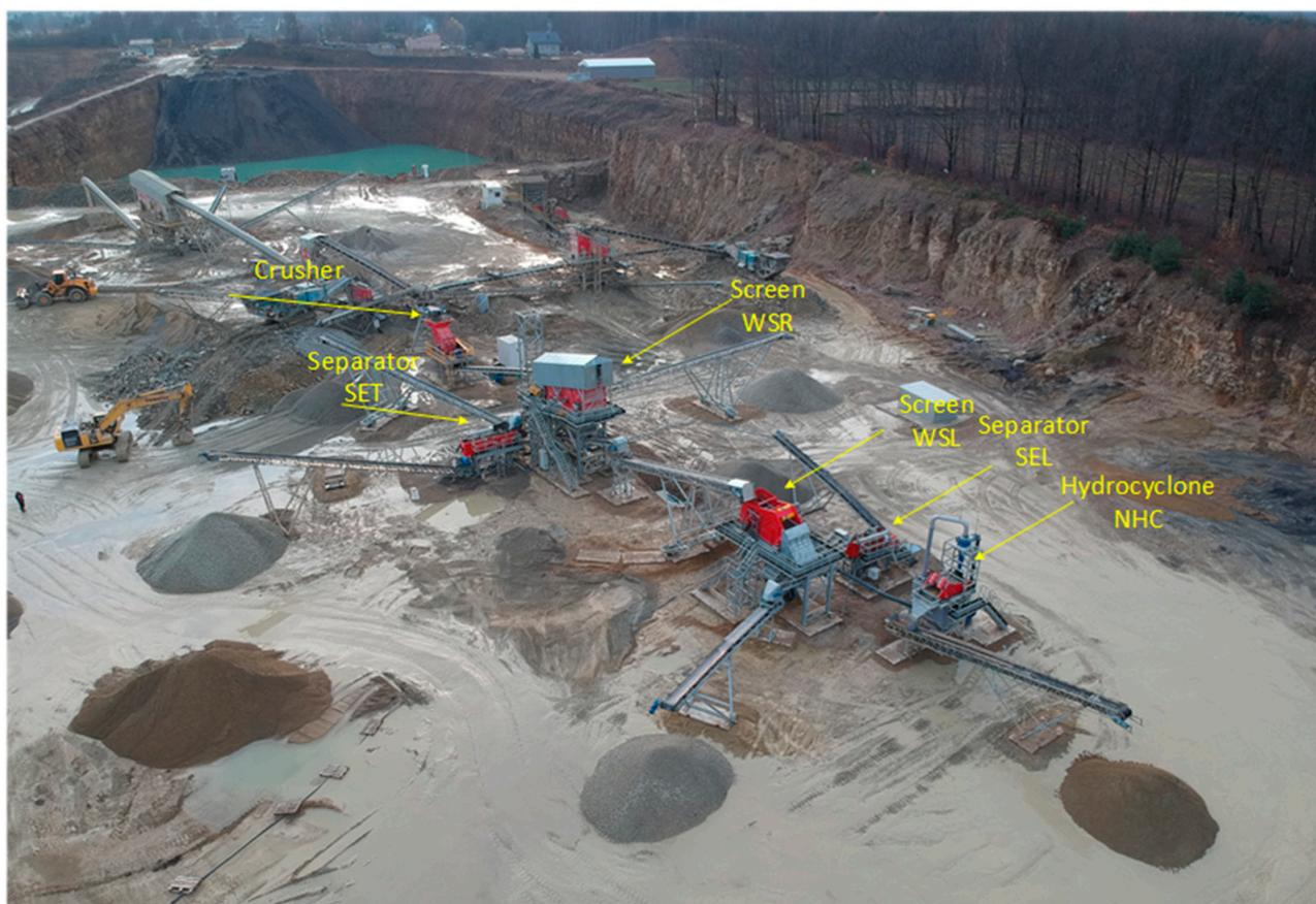
**Figure 1.** Technological line in the Imielin Dolomite Mine, image from a drone.
