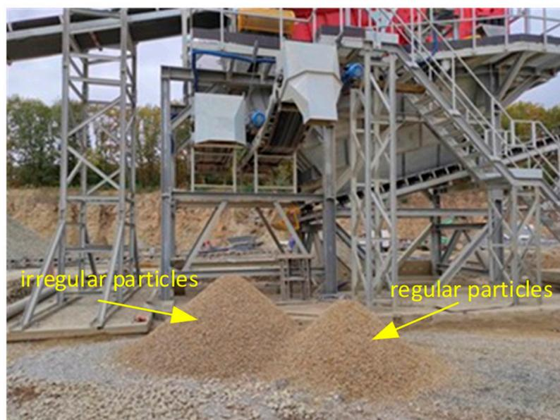
**Figure 6.** Limestone tests 8–16 mm regular and irregular particles.
