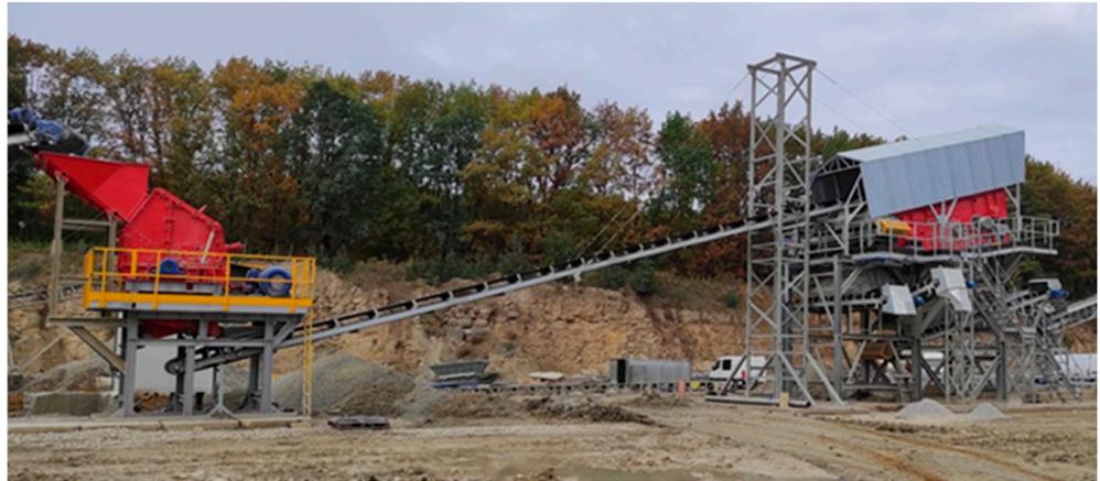
**Figure 3.** View of the KU 80/120 crusher and the WSR 3-2.0/6.0 screen.
