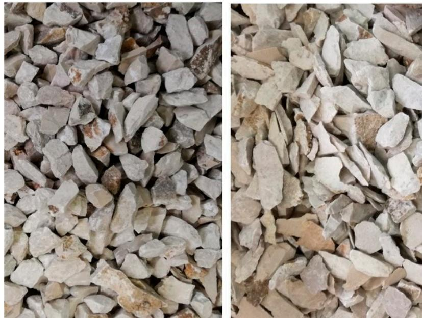
Figure 8. Final product: Limestone 8–16 mm regular (left), irregular (right).
