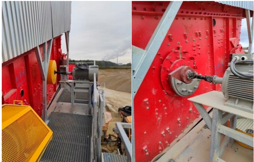
Figure 11. Change of unbalanced masses on the eccentric shaft of the screen.
