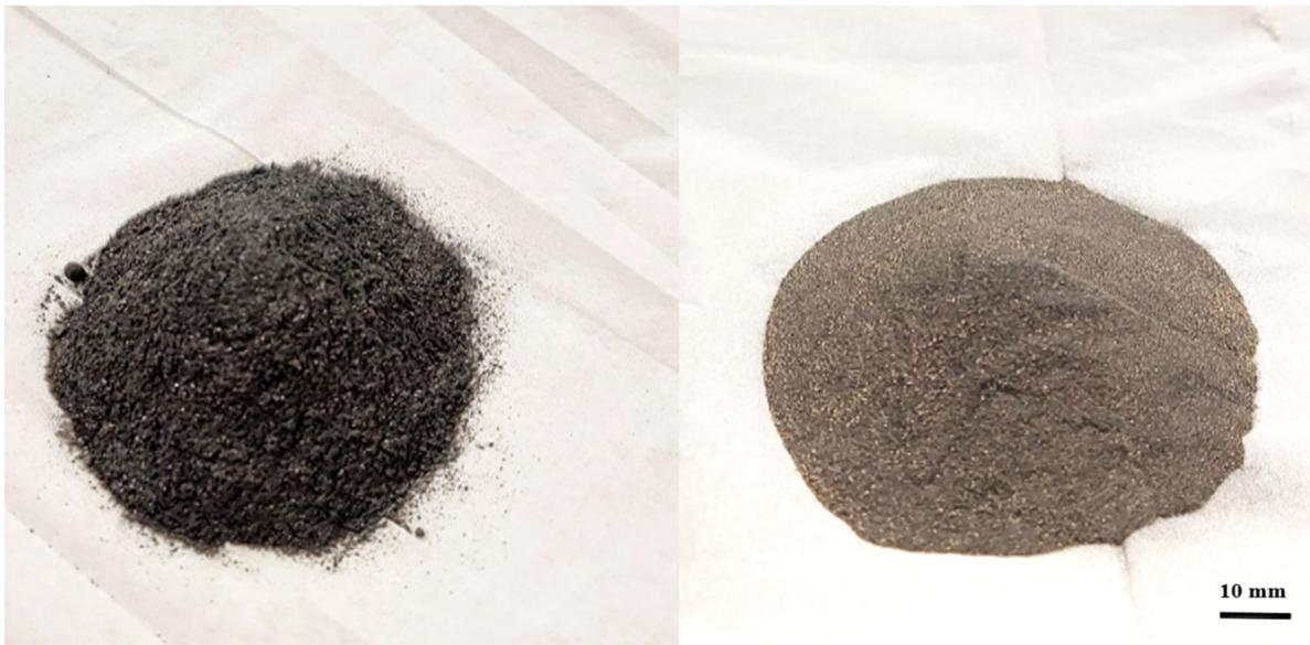
**Figure 3.** Ilmenite sand (left) and grinded material (right) from the Metchib company, Quebec, Canada.
