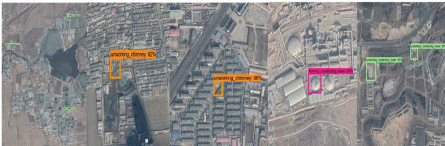
Figure 5. The false detection objects are divided into five categories: lake, road, architecture, tank, and other objects. The pink boxes represent working condensing tower, the green boxes represent non-working condensing tower, and the yellow boxes represent non-working chimney.
