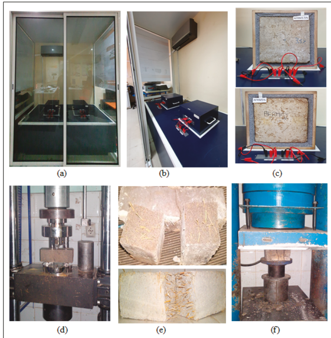
Figure 4. Devices used for thermo-mechanical tests: (a) air conditioned chamber, (b) two boxes method, (c) boxes of measured thermal conductivity and diffusivity, (d) flexural test, (e) two half prisms obtained from flexural test and (f) compressive test.
