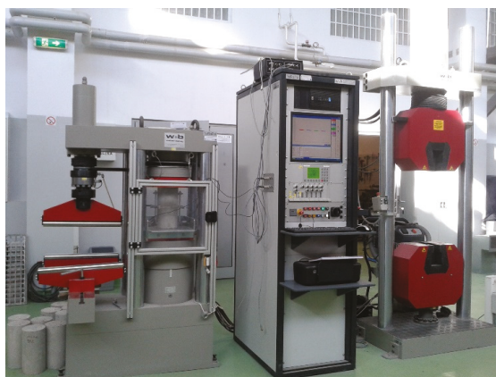
Figure 1. The test stand for testing the static modulus of elasticity.
