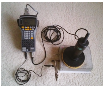
Figure 3. The connection scheme of the GP-5000 GalvaPulse™ set with the tested reinforcement.
