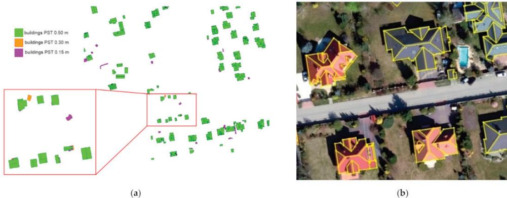
**Figure 5.** LiDAR rooftop polygons: (a) adjustment of the Plane Surface Tolerance values, (b) selected examples of building rooftop outlines (yellow lines) superimposed on aerial orthoimagery.
