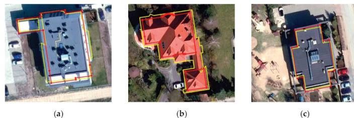
**Figure 12.** Building outlines: yellow from LiDAR, red from the cadastre: (a) multi-family building extracted as two building outlines; (b) two connected single-family houses denoted by LiDAR as one building; (c) outlines of a kindergarten.
