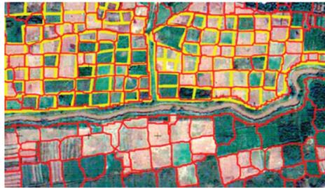
**Figure 10.** Nyandwai et al.'s method [281] created a 'first cut' cadastre (yellow) that could be taken to the field for validation.
