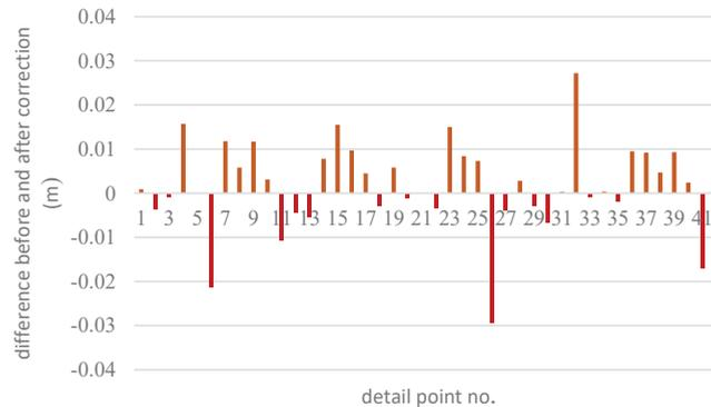
**Figure 30.** Error difference of digitized detail line data using the corrected and uncorrected handheld LiDAR point clouds.
