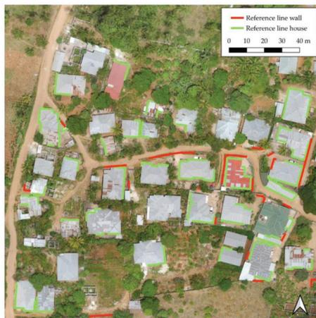
**Figure 8.** Selected reference lines representing rooftops (green) and walls (red) for the area of interest in Kibonde.
