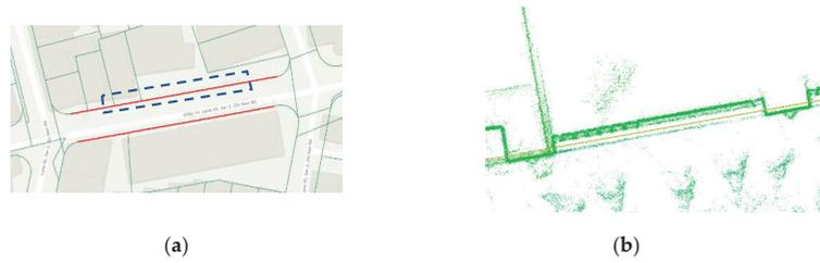
**Figure 23.** Possible cadastral detail line on an existing road boundary. (a) The digitized possible cadastral lines. (b) Overlap of point cloud and the cadastral map.
