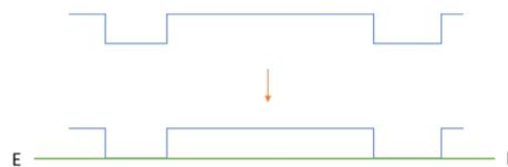
**Figure 25.** The digitized process of the possible cadastral line close to the road boundary.
