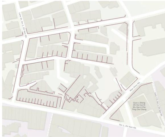
**Figure 26.** The result of digitized detail lines from the corrected handheld LiDAR point cloud.
