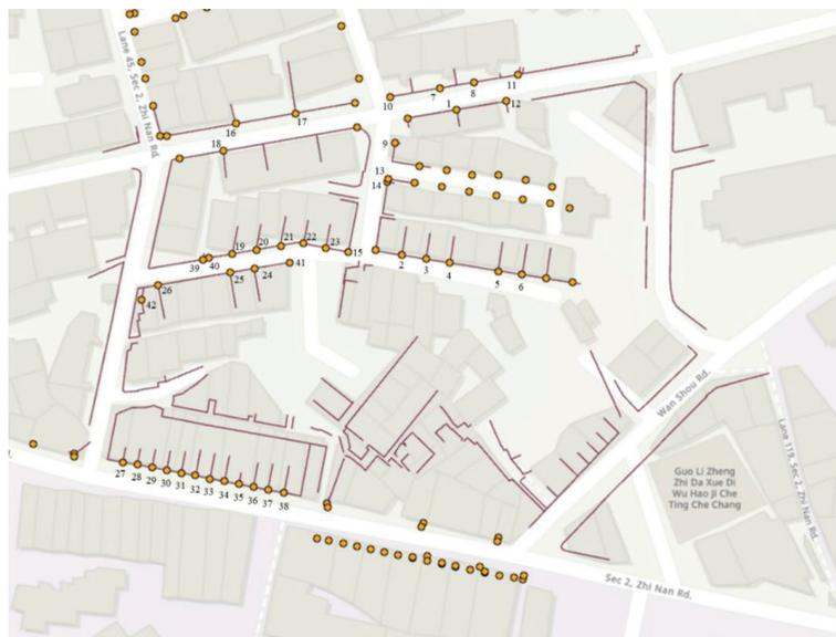
**Figure 27.** The digitized results of the corrected handheld LiDAR points and detail points surveyed by a total station.
