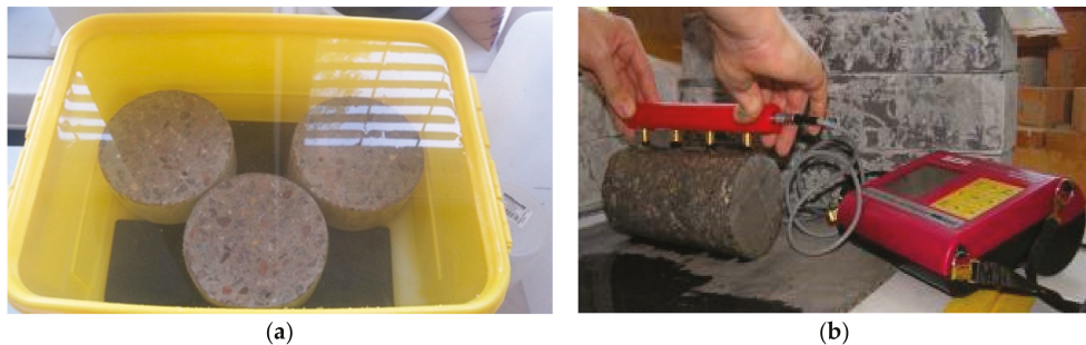
Figure 4. Specimens in chloride solution prepared for NT BUILD 443 test (a) and diffusion coefficient testing based on AASHTO TP-95 (b).
