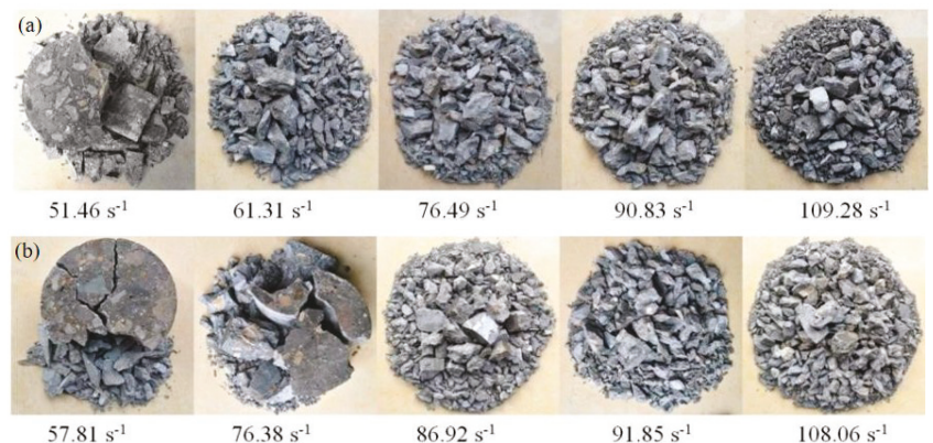
Figure 10. Typical failure mode of concrete under different strain rates (a) PC; (b) CNFC02.
