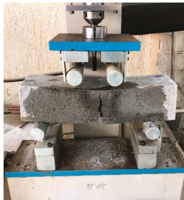
Figure 5. Third-point loading test to obtain the modulus of rupture.
