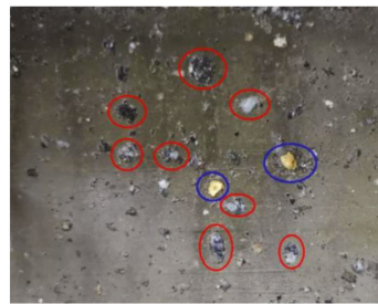
Figure 7. Typical photo for damage of aggregate in specimen FIG2A1-2 (red circle: coarse aggregate; blue circle: fine aggregate).
