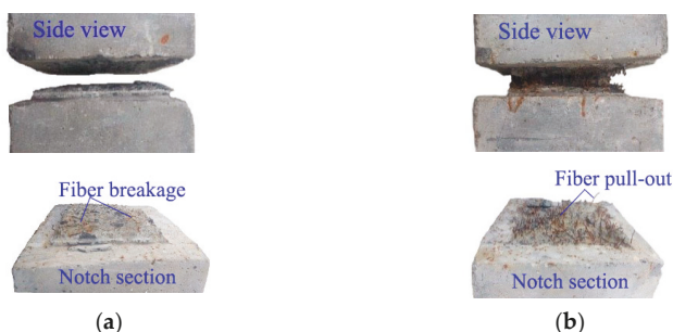
Figure 6. Typical failure patterns of axial tensile specimens: (a) fiber breakage of HFb04; (b) fiber pull-out of HFb12.
