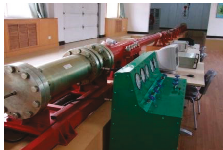
Figure 3. \Phi 100 mm SHPB test system.
