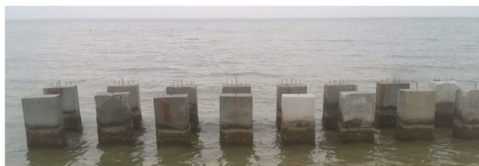
Figure 1. Concrete blocks setup in the tidal zone (inner blocks: reinforced; outer blocks: plain).
