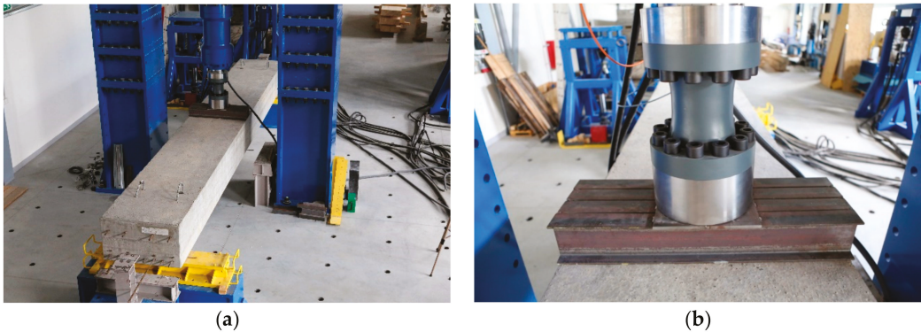
Figure 8. Three-point loading test in Centre of Building Experiments (a), and spreading of concentrated force with steel element (b).
