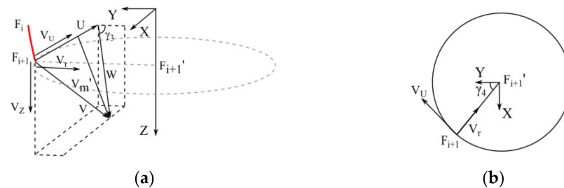
Figure A6. Diagram of the velocity triangle and decomposition: (a) spatial sketch; (b) top view.
