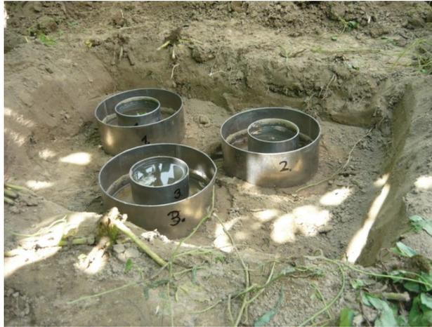
**Figure 2.** The double-ring infiltrometer (DRI) (photo. L. Borek).
