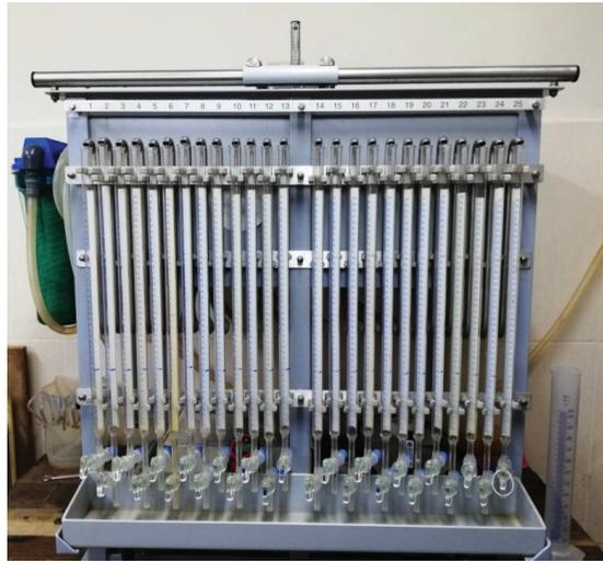
**Figure 3.** The laboratory permeameter produced by the Eijkelkamp (photo. Ł. Borek).
