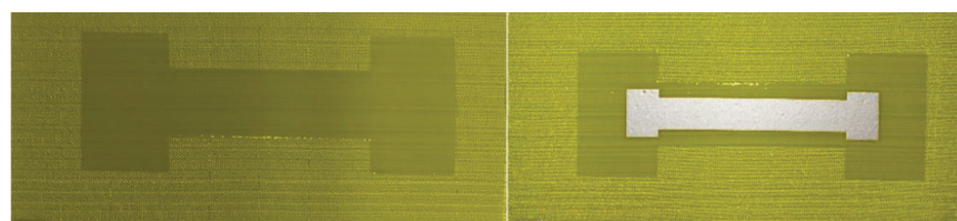
Figure 3. Screen-printed dumb-bell interface (left) and silver conductor (right) patterns on a bespoke woven Isacord Polyester 60 thread count (IsacordPoly60) fabric.
