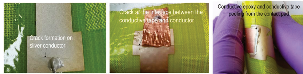
Figure 5. Crack formation on samples with bonded joints conductive epoxy ( left ), pressure bonded conductive film ( middle ) and epoxy + conductive film ( right ).
