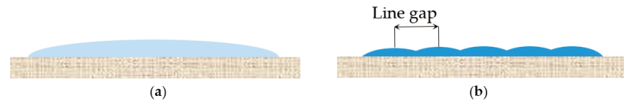
Figure 3. The effect of line gap on printing result. (a) The cross-section of a printed track achieved by one wide print. (b) The cross-section of a printed track achieved by five narrower prints.
