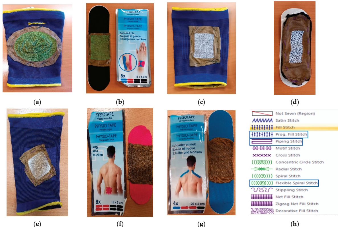
Figure 1. This figure shows the different body movement sensors with compression sleeves, physio tape and selection of four stitch types that give the maximum flexibility of movement (a) knee sensor with knee bandage; (b) knee sensor with physio tape; (c) elbow sensor with elbow bandage (d) finger movement sensor (e) elbow sensor with piping stitch and rhombus shape for maximum flexibility of movement (f) back movement sensor with physio tape (g) shoulder movement sensor with physio tape (h) selection of stitch types (Fill, Prog. Fill, Piping, and Flexible spiral stitch).
