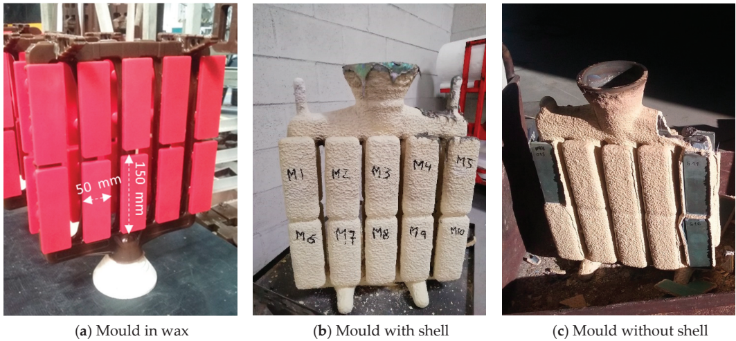
Figure 1. Investment casting moulds in different manufacturing steps.
