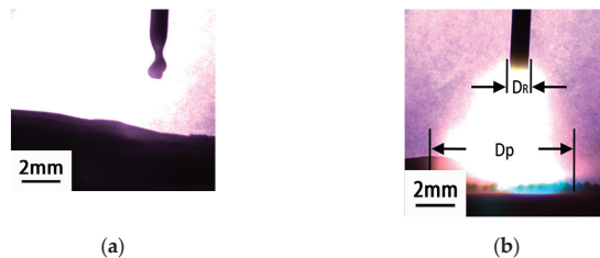
Figure 5. (a) Complete filtering out of the arc; (b) typical nature of arc profile.
