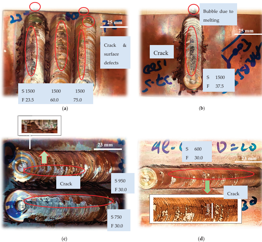
Figure 11. Dissimilar Cu-2219 Al lap joints fabricated by WC square-tool.
