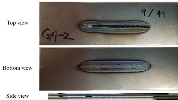
Figure 6. Workpiece appearance with a gap of 0.8 mm after welding with a welding speed 1.5 m/min and a laser power of 3000 W: top view, bottom view, side view.
