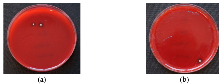
Figure 4. Examples of Staphylococcus aureus on Columbia agar. (a) Polyether Adhesive (PA) after 15 min incubation; (b) Polyether Contact Tray Adhesive (PCTA) after 30 min incubation. In Universal Adhesive (UA) and Fix Adhesive (FA), no colonies could be detected at both times.
