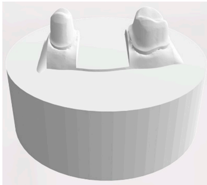
Figure 5. Design of the object holder with two prepared teeth.
