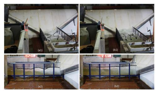
Such concentration of the flow at the center of the basin generates lateral flow toward the sidewalls that spreads downstream (Figure 11a1).
