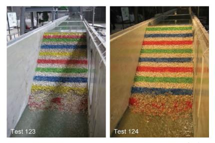
**Figure 17.** Failure progress in tests n<sup> $\circ$ </sup> 123 and 124 for a discharge of roughly 0.0090 m<sup>3</sup> s<sup>-1</sup>.
