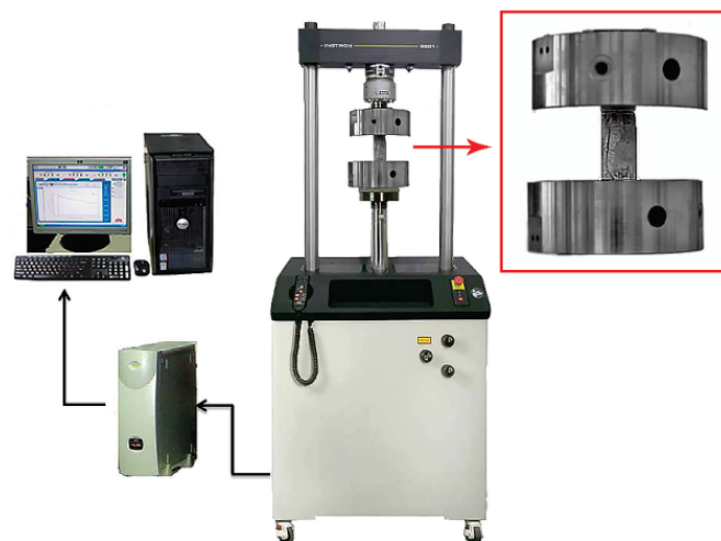
Figure 5. Experimental apparatus for compressive stress test (close up shows a fractured sample).
