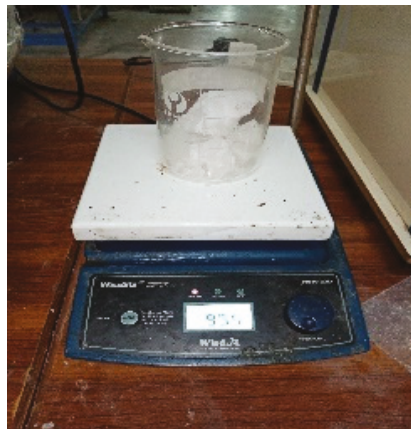
Figure 1. Magnetic stirring of samples in the beaker placed on a hot-plate heater.
