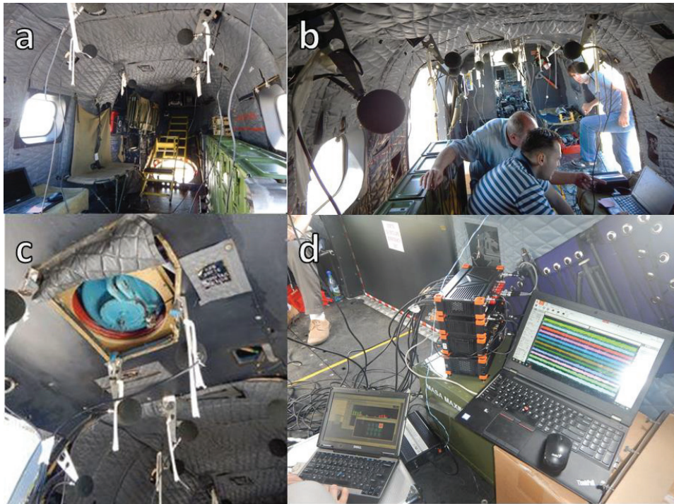
Figure 4. The locations of the microphones in the helicopter and the measurement equipment: (a) microphones from A5, A6, A7; (b) microphones from A1, A2, A3, A4; (c) microphones under transmission gear A3; (d) measurement equipment.
