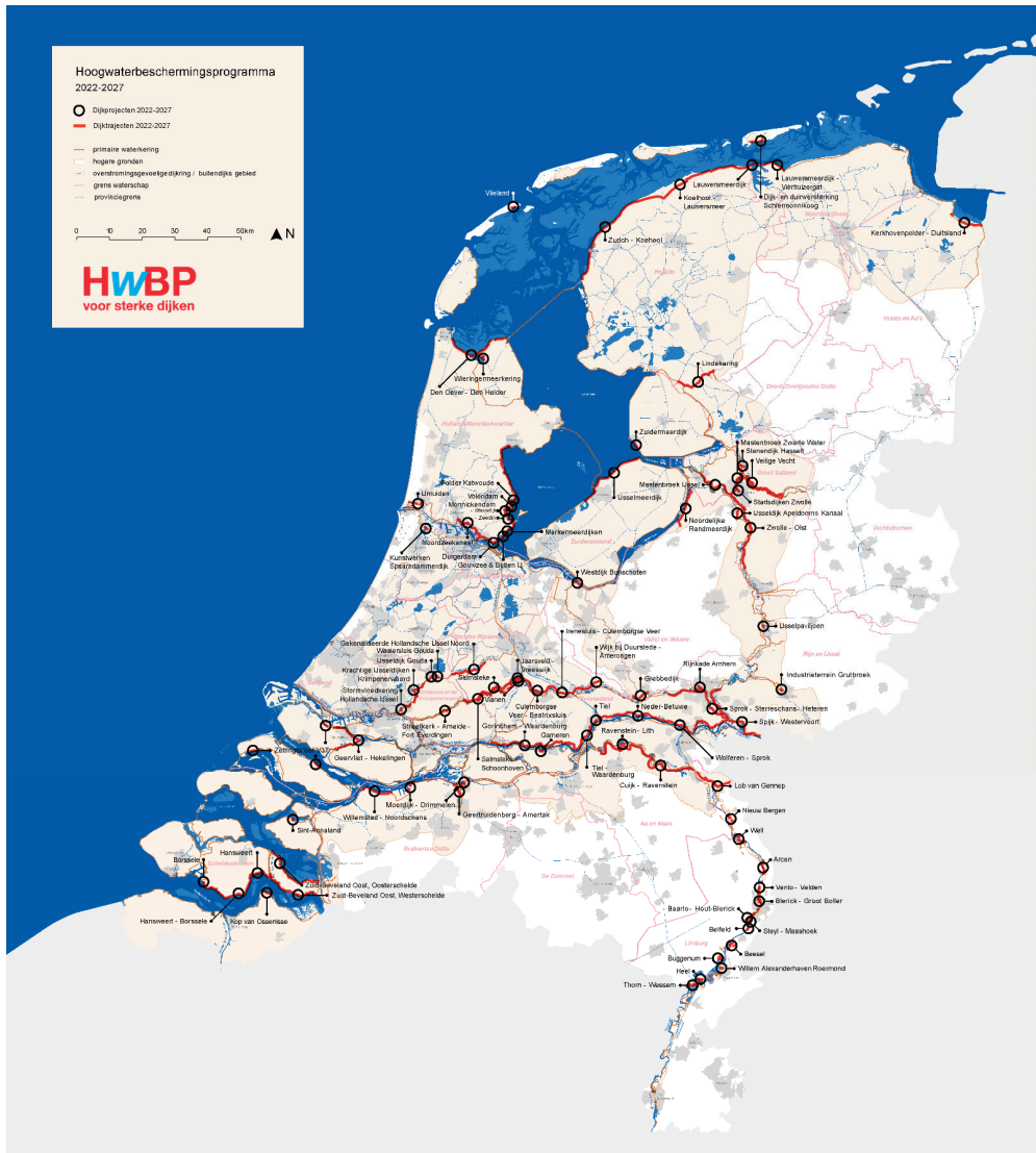
Figure 1. Current scope of projects in the Dutch Flood Protection Programme until the year 2027. The expected scope until 2050 is about 1500 km of dikes and about 500 civil-engineering structures.
