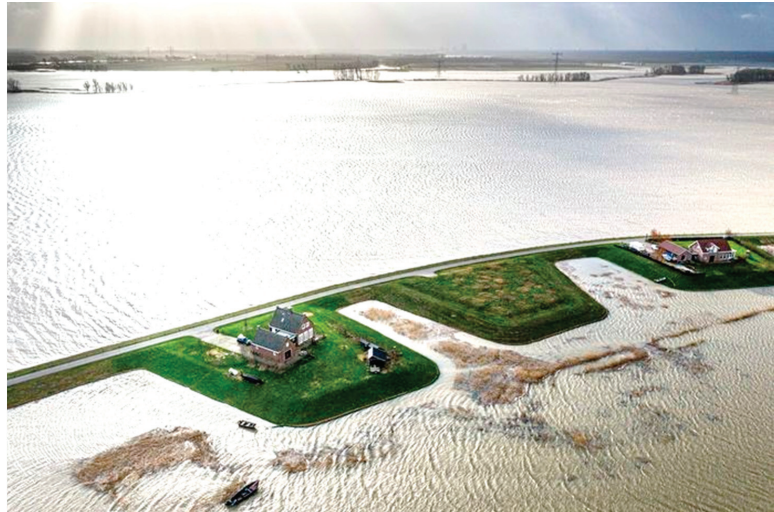
Figure 6. Relocated houses on flood-free mounds in Noordwaard flood storage and bypass area (picture from Brabants Dagblad).
