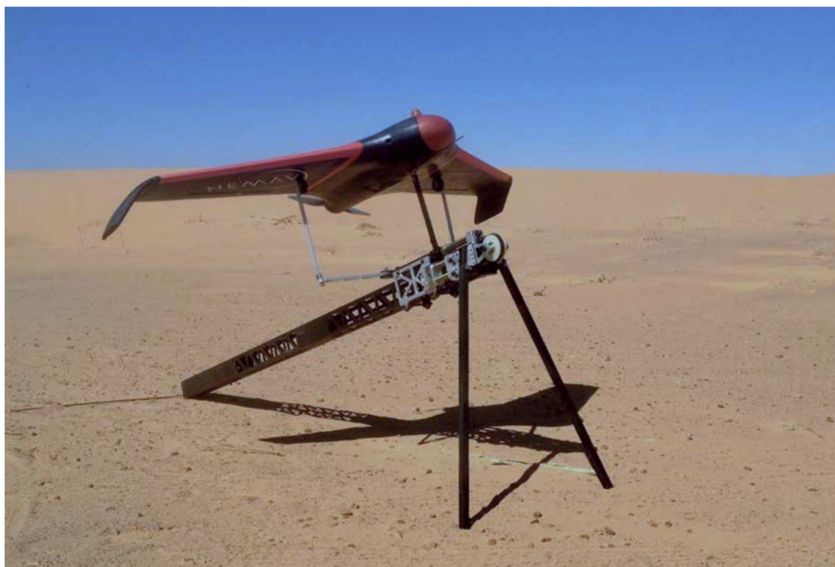
Figure 2. Fixed wing drone for desert locust monitoring (source: FAO [24]).
