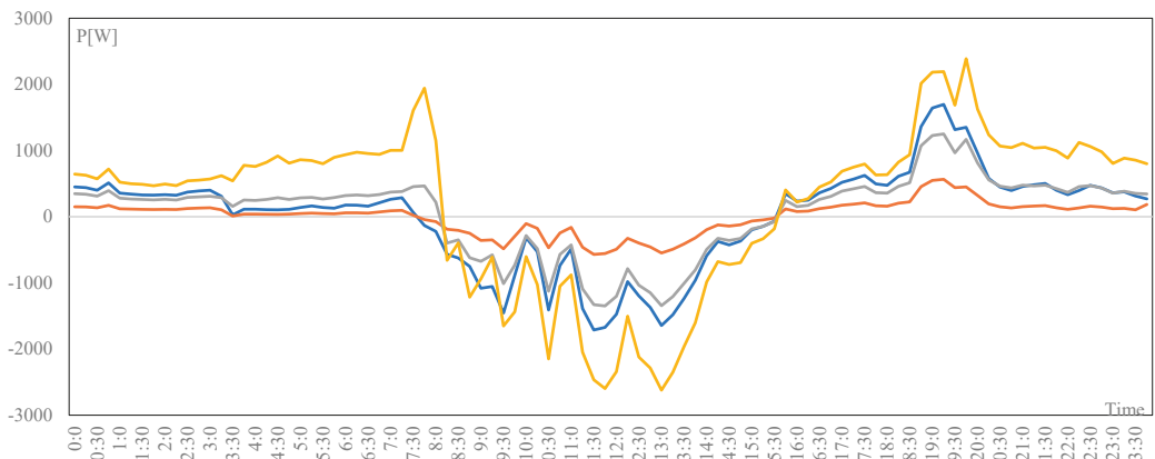
Figure 22. Exchanged power with the storage system for the different AEU: AEU1 (blue), AEU2 (orange), AEU3 (grey), AEU4 (yellow).
