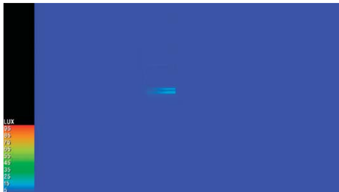
Figure 7. IESVE illuminance simulation for corridor A in the current situation, illustrating lux levels below 3 lx.
