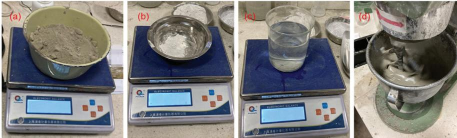
**Figure 4.** Preparation process of the filling slurry sample. (a) Weigh tailings of a certain mass, (b) weigh cementitious materials of a certain mass, (c) weigh some water, (d) pour the tailings, curing material and water into the hopper of the mixer successively and mix for 10 min at 60 r/min to evenly distribute the components.
