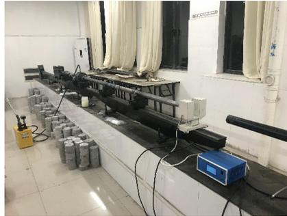
**Figure 1.** SHPB test system.
