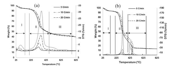
Figure 2. Thermograms of mass loss and mass-loss rate (DTG) for GG in (a)  $N_2$  and (b) air atmospheres.
