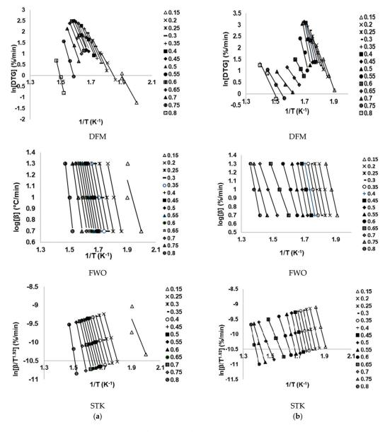
Figure 4. Plots of linear curves for DFM, FWO, STK models in (a) N<sub>2</sub> and (b) air environments.
