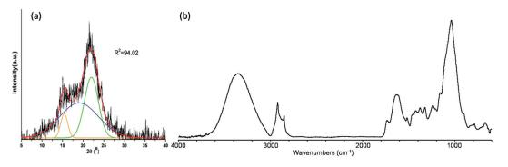
Figure 1. (a) X-ray diffractogram and (b) FTIR spectrum of guinea grass.
