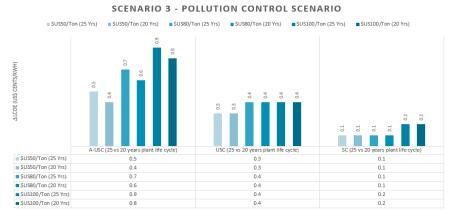
Figure 7. Scenario 3: LCOE differences between HELE and subcritical technologies for different coal prices and economic life span of the plant.
