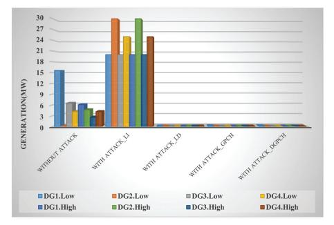
Figure 9. Production of distributed generation sources (DGSs) in different scenarios.
