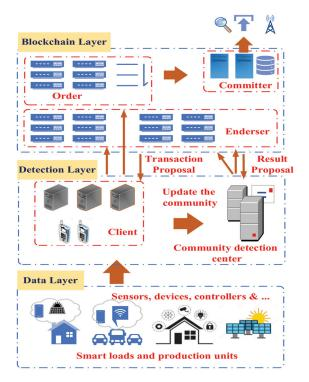
Figure 1. The data-sharing structure according to the blockchain technology.
