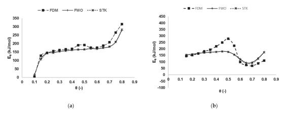
**Figure 5.** Plots of apparent activation energy,  $E_{\theta}$ , against conversion ratio,  $\theta$ , (**a**) N<sub>2</sub> and (**b**) air environments.
