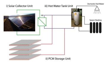
Figure 2. Diagram of a solar energy and latent heat thermal energy storage (S-LHTES) system with phase change material (PCM). Adapted from Englmair et al. [19].
