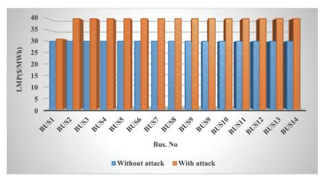
Figure 6. LMPs at different buses in the case of an incremental load attack.
