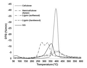
Figure 3. Thermograms of mass-loss rate (DTG) of cellulose, xylan, lignin, and GG in  $N_2$  atmosphere at 20 °C/min.
