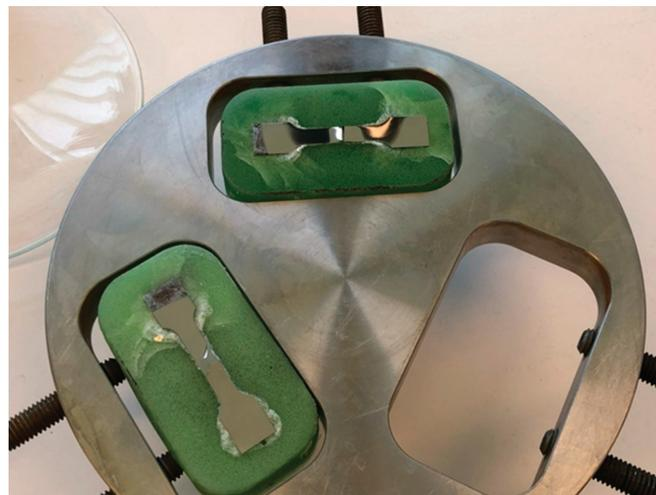
**Figure A1.** Specimens after polishing in Technovit-5071.
