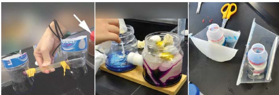
Figure 3. MFC prototypes by Group G. From left to right: first prototype, arrow indicates “fermentation MFC” made by Gerald at home and brought to class; second prototype made at home by Gerald, with inflated latex gloves and pebbles used to displace volume; incomplete third prototype made during final MFC Challenge session.
