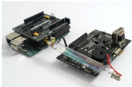
Figure 3. Raspberry Pi and Geiger Sensor (left) connected to the Bridge board and the Geiger Sensor board (right).
