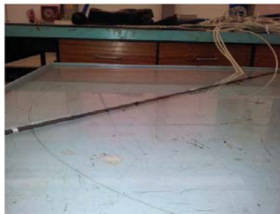
Figure 7. Sealing testing with sensors immersed in water.
