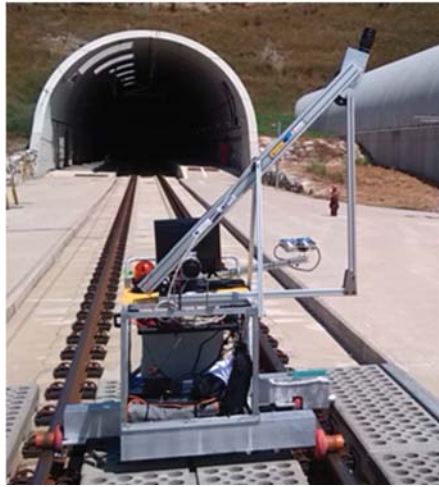
Figure 5. Prototype of the tunnel inspection platform.
