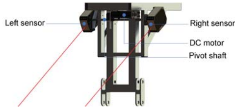
Figure 5. Scanning system positioned on the SCMS frame.
