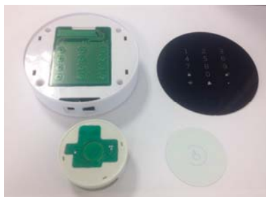
Figure 9. Image of the base station and gas sensor, and packing design.
