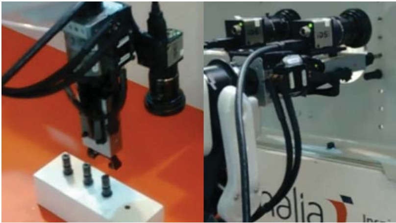
Figure 9. (a) The right arm of the robot is taking a rivet from a tray; (b) after taking the rivet, it is introduced in the previously-detected drilled hole.
