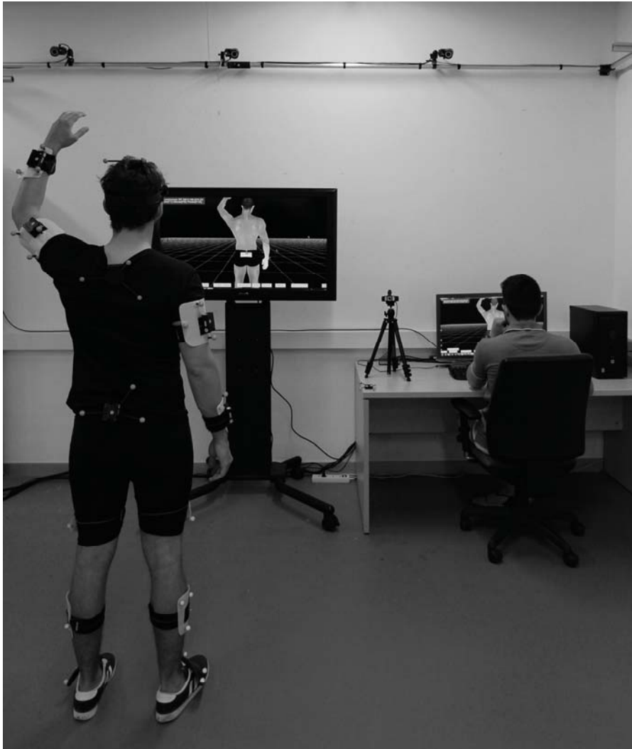
Figure 2. MoCap service, biomechanics laboratory. System with simultaneous optical and IMU technology (optical full body MoCap and IMU upper body MoCap).
