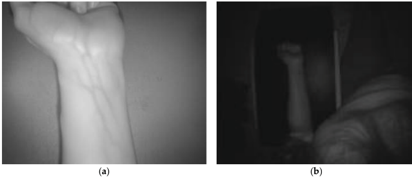
Figure 7. Test 2 - Acquired images. (a) SWIR image; (b) TOF amplitude image.
