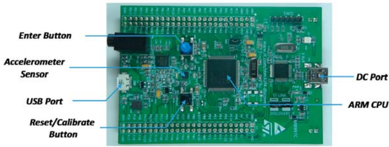
Figure 8. Data acquisition system based on the STM32F4-Discovery board.
