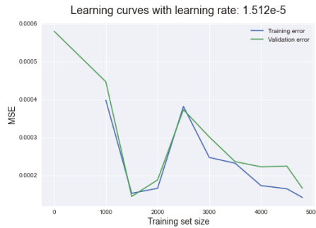
Figure 11. Influence of the training set size in the training and validation phases for the inverse biaxial test model.
