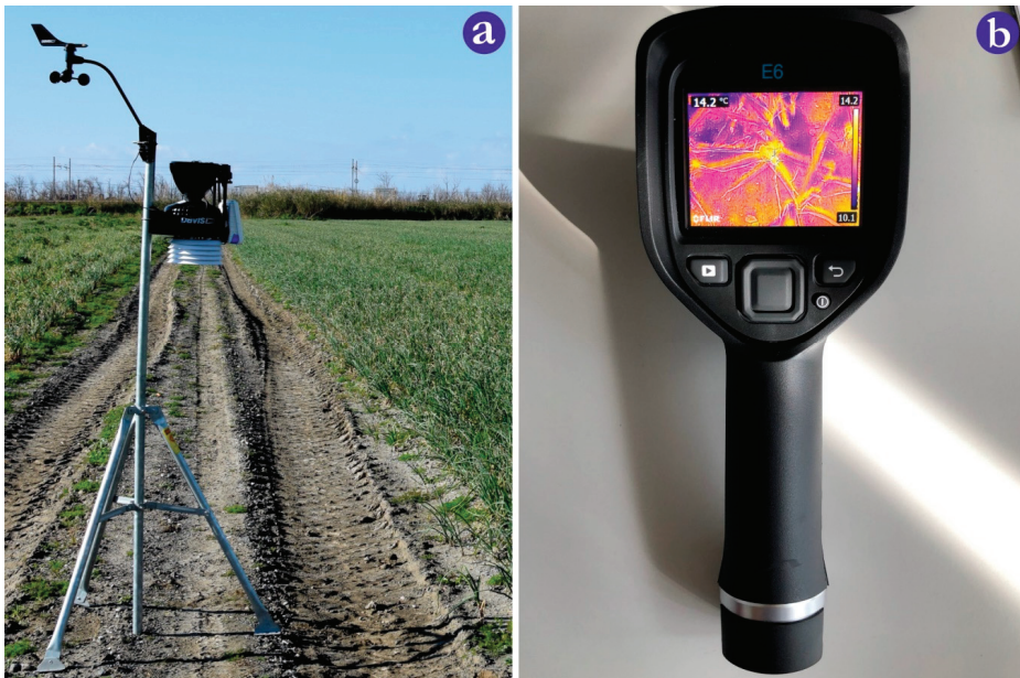
Figure 6. (a) The weather station used during the thermal surveys on an onion field. (b) Handheld infrared thermometer used to measure the temperature of reference surfaces (photos taken by the authors).
