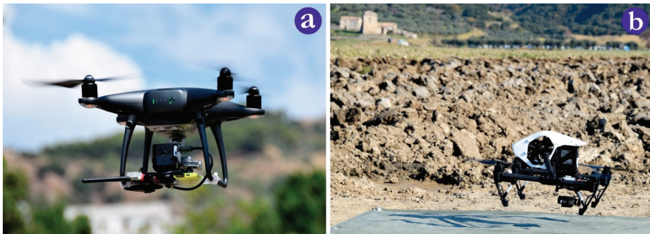
Figure 3. DJI Phantom 4 pro (a) and (b) DJI Inspire 1, both equipped with a FLIR uncooled thermal camera (photos taken by the authors).
