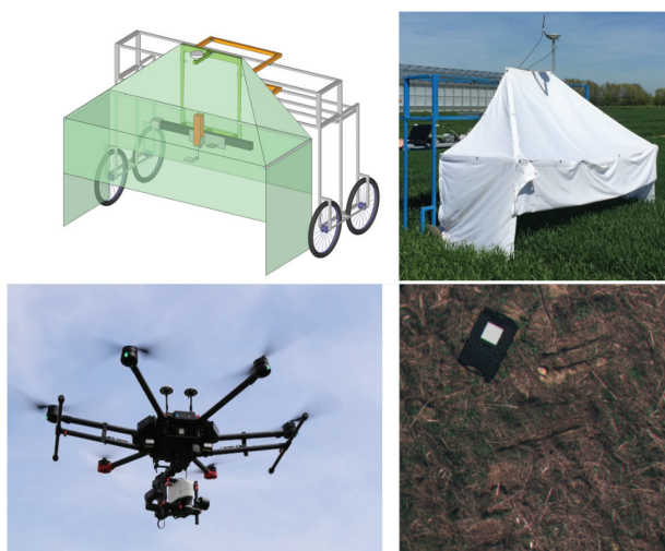
Figure 3. Construction plan of the Phytobike ( top left ) and the final appearance in the field including the cotton diffuser ( top right ). The UAV system used, consisting of a DJI Matrice 600 and a Rikola hyperspectral camera ( bottom left ). Normalization was performed using a 50% grey reference panel ( bottom right ).
