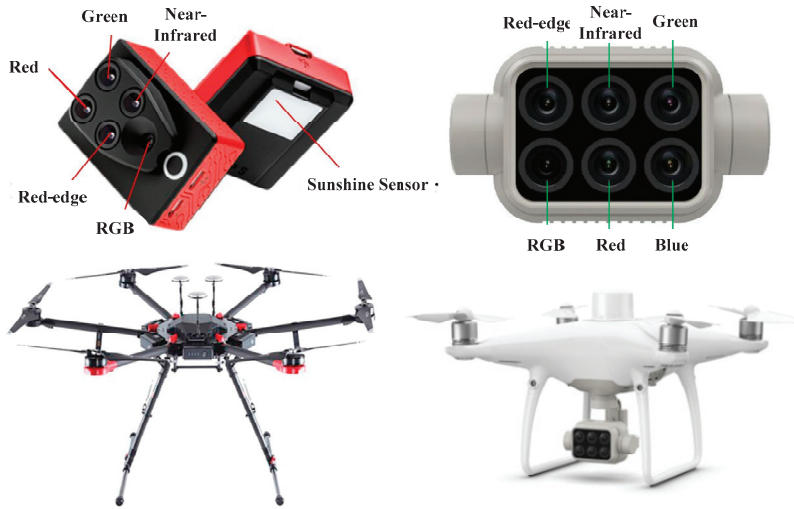
Figure 2. UAV platforms and multispectral sensors (Sequoia and P4M). The Sequoia sensor is carried on the EM6-800 hexarotor UAV (left), and the P4M uses its own aircraft (right).
