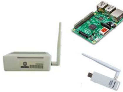
Figure 4. Listening device used in the people flow monitoring sensor network.
