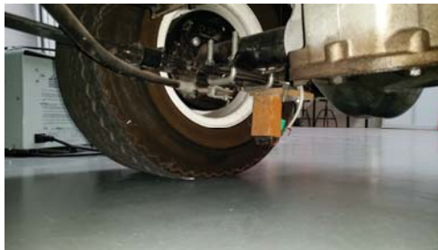
Figure 5. Range sensor used to get a real time radius measurement used to improve odometry accuracy.
