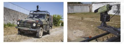
Figure 5. Vehicle-mounted color camera system.
