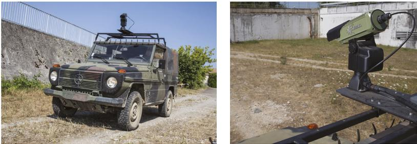
**Figure 5.** Vehicle-mounted color camera system.
