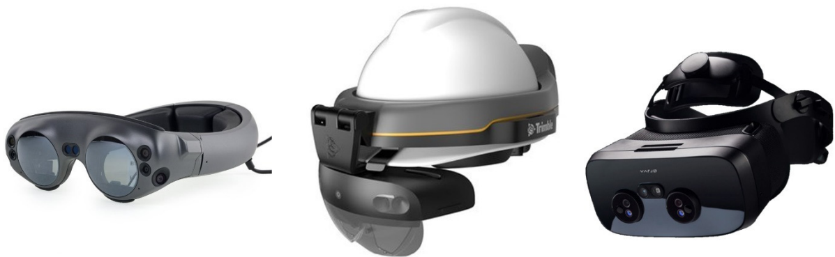
Figure 4. Magic Leap 1 (left), MS HoloLens 2 on Trimble (Sunnyvale, CA, USA) XR10 (center), and Varjo XR-3 (right).
