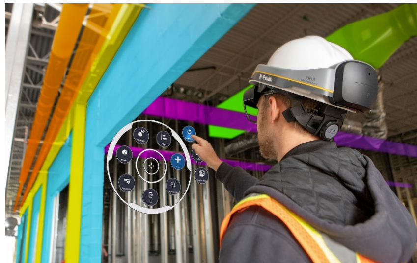
Figure 9. Example of Trimble XR10 MR application on construction site.
