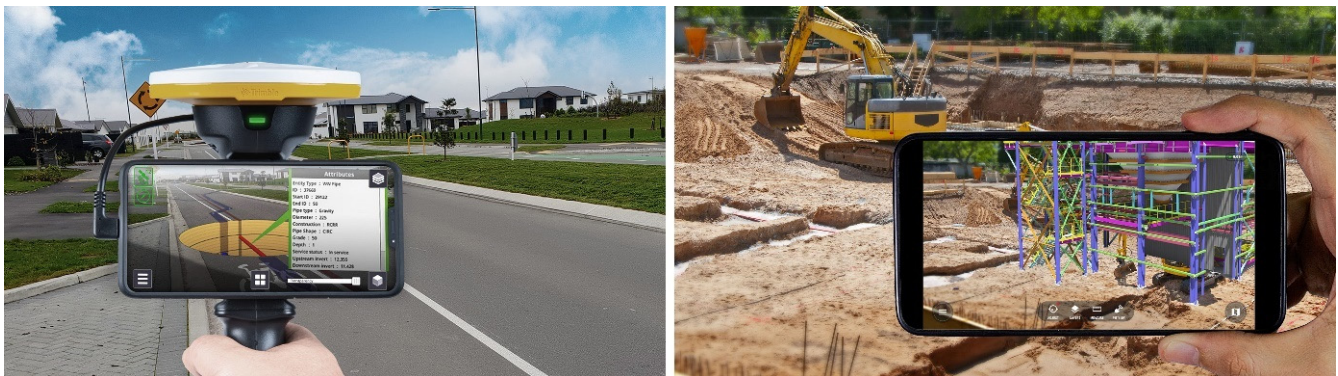
Figure 5. Trimble SiteVision AR system (left) and smartphone-based AR (right).
