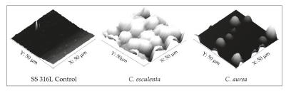
Figure 1. AFM images of a polished SS 316L (control) plate, C. esculenta and C. aurea leaves.
