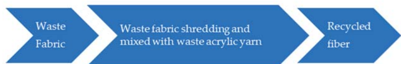
Figure 1. Steps to recycle waste fabrics.
