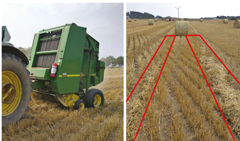
Figure 5. The narrow pick-up of the round baler (left) caused high loss of straw (right) along the swath (areas of the swath not reached by the baler's pickup system are highlighted in red).
