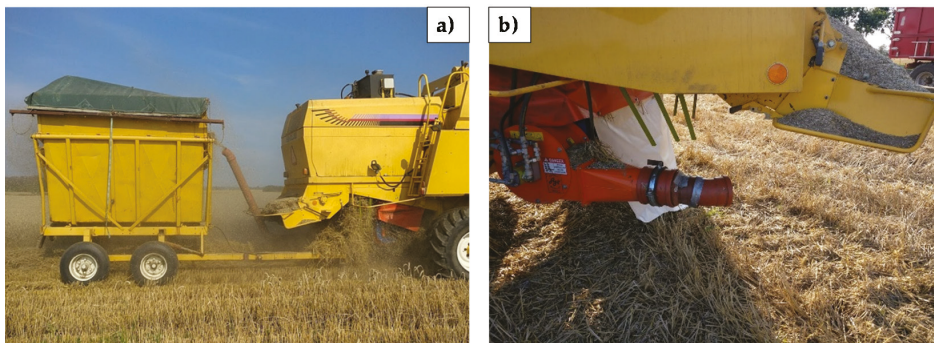
Figure 3. (a) Loose in a towed trailer (CoT) = chaff recovery system mounted in New Holland TX68, for the discharging of the product on a towed trailer (Trailer Agrohill Maskin AB, Halmstad, Sweden); (b) CoS = chaff recovery system mounted in New Holland TX68, for the discharging of the product on top of the swath.
