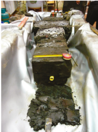
Figure 6. The coal blocks cemented to each other by a mixture of gudron (Source: own elaboration).
