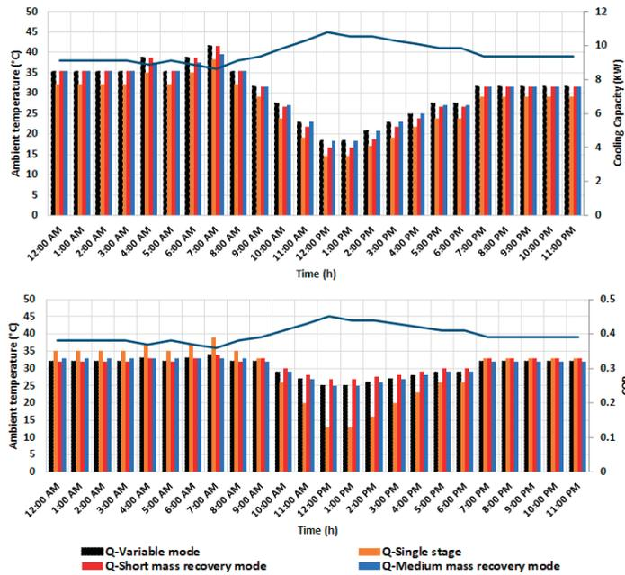
Figure 21. Measured ambient temperature and expected cooling capacity and COP for various modes (day 1).
