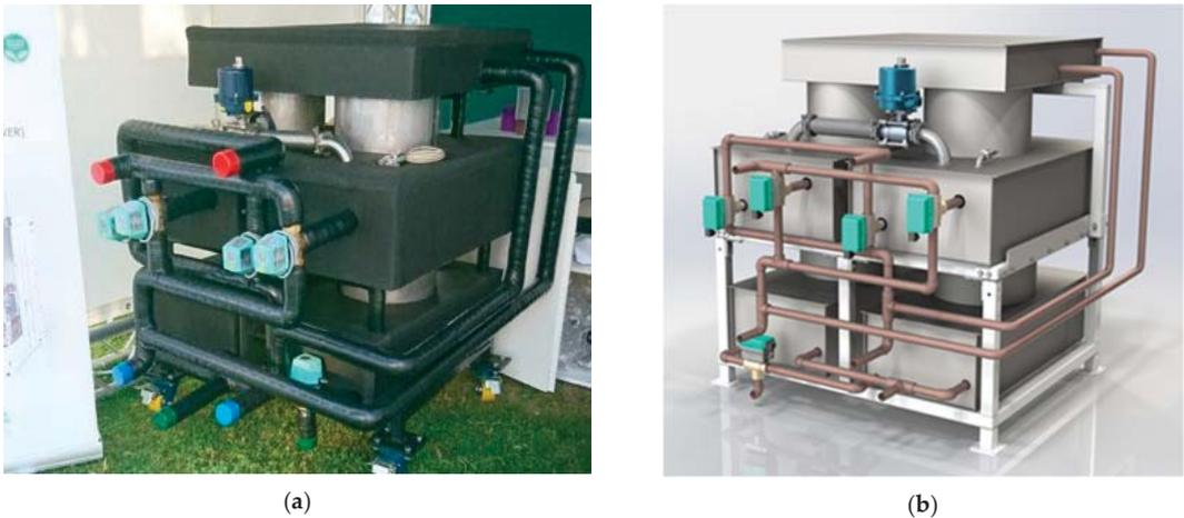
Figure 7. PI prototype adsorption chiller: (a) prototype, (b) 3D model.
