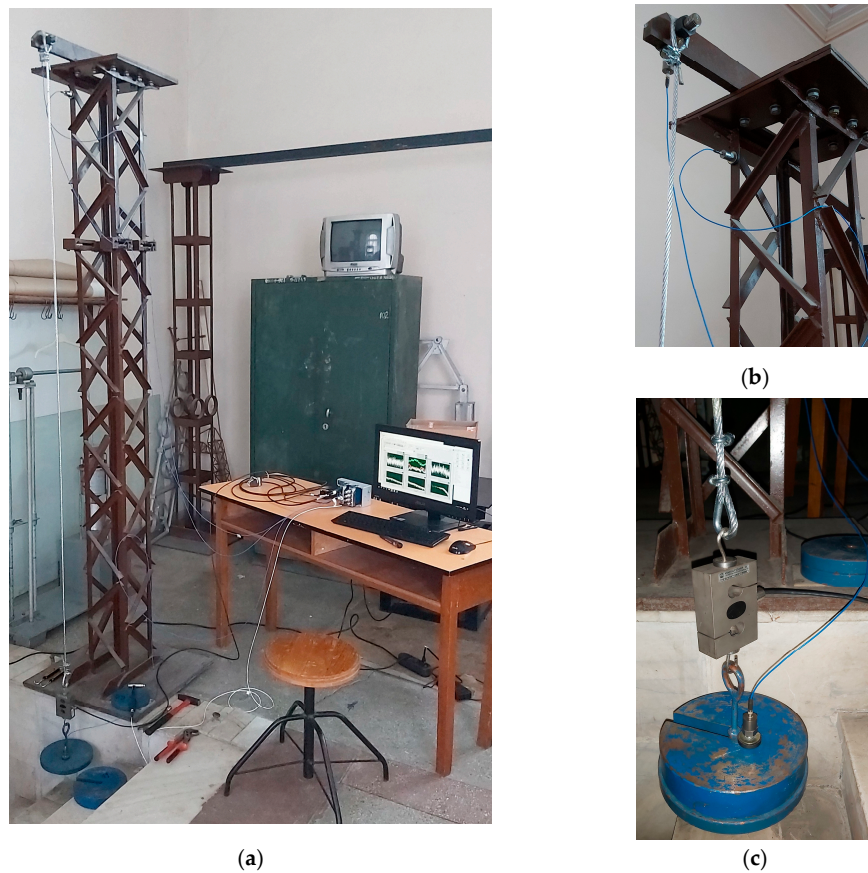
Figure 1. The laboratory experimental setup: (a) General view with a latticed tower, wire rope sample, static charging device, and compute-based acquisition system; (b) detailed view of the upper side of the tower, with the hung rope device and residual motion monitoring transducers; (c) detailed view of the wire rope charging device with an additional mass applied and transducers for monitoring the forces and oscillations, respectively.
