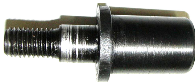
Figure 2. Constructive shape of bolts.
