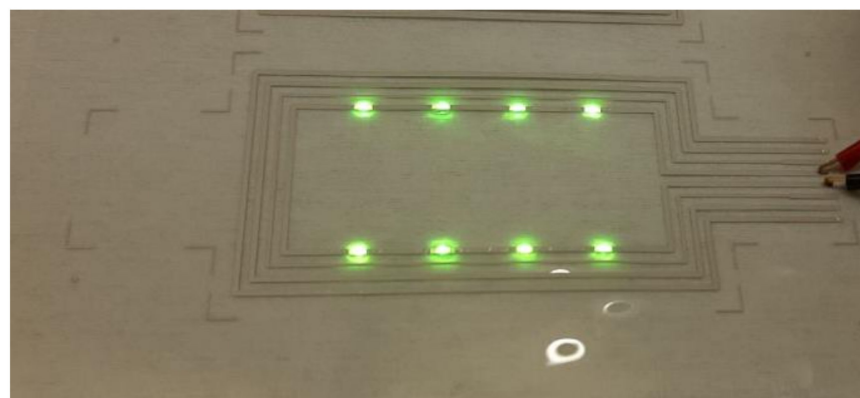
Figure 8. Screen-printed hybrid-integrated LED foil.
