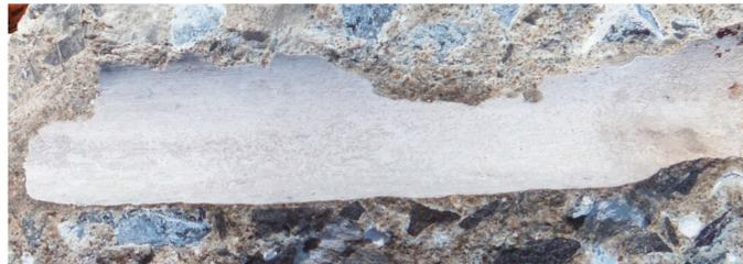
**Figure 5.** Example of high quality, well-compacted concrete broken open after more than 80 years of continuous marine exposure, showing the void-free surface that interfaced with the steel 32 mm diameter reinforcing bar (removed for clarity). No corrosion was detected along the whole 5–7 m of reinforcement bar (photograph © RE Melchers, 2020).
