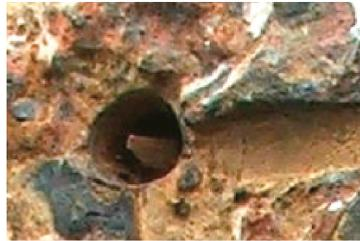
**Figure 8.** End view of remains of 32 mm diam. reinforcement bar, with watery-looking rust stains on a cracked concrete cross-section, after 85 years of exposure to seawater in tidal conditions (photograph courtesy of Clayton Smith).
