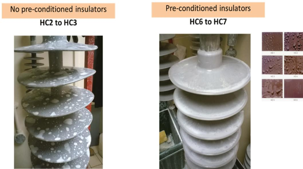
**Figure 4.** Examples of the effect of pre-conditioning on the HC index.**Table 2.** Characteristics of the used insulators.
