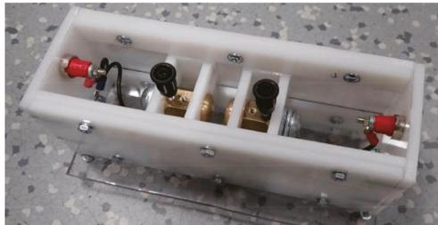
Figure 9. Adjustable sphere–sphere spark gap [33].
